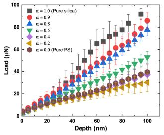
Fig. 7 The measured load versus depth data, averaged over data for 5-6 different locations on the film, is plotted as a function of  $\alpha$ . As the fraction of hard particles increases, the slope increases. Discrepancy was observed for  $\alpha = 0.2$ , which had the lowest slope.
