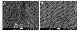
SEM images of the surface of a film containing equal volume of soft and hard particles ( $\alpha = 0.5$ ). (A) The image shows a crack at the edge of the film. (B) The image shows a crack-free region in the interior of the film. Note that in all cases, both the PS and silica particles retained their spherical shape indicating pure elastic deformation of the particles.
