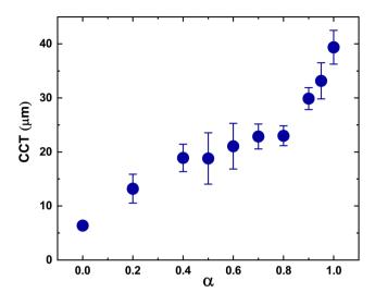
Fig. 4 The measured critical crack-free thickness versus fraction of hard particles ( $\alpha$ ). The CCT was determined using images from microscopy and thickness profiles from profilometry. Films with softer particles crack at lower thickness (low CCT)
