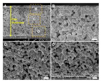
Fig. 2 Particle distribution in the dried particle film at  $\alpha$  = 0.5. The dried film was heated up to 200 °C for 60 min to allow the PS particles to deform. These images show that the silica particles remain spherical while the PS particles are completely deformed. The first image on the top left (A) is the entire cross-section of the film, while the enlarged images of sections B, C, and D at various depths are shown in the remaining images.
