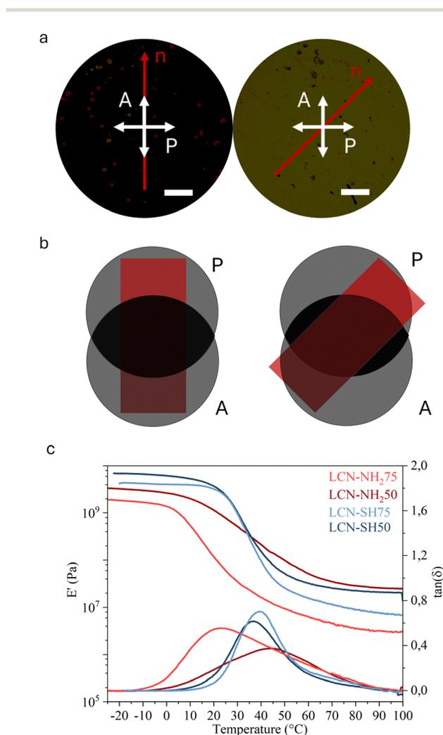
Fig. 2 Molecular alignment and mechanical tests on LCN films. (a) POM images of an LCN film with the director ( $n$ ) oriented orthogonally to the polarisers and at 45°. Scale bar: 200  $\mu\text{m}$ . (b) Schematization of the transmittance of LCN films under two crossed polarizer ( $P$ ) and analyser ( $A$ ). (c) Storage modulus ( $E'$ ) and  $\tan(\delta)$  representative curves for the LCNs synthesised.
