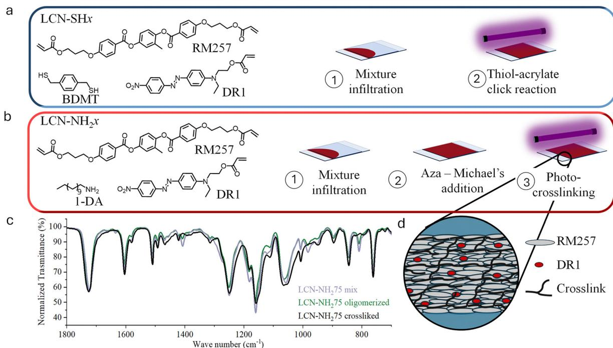
**Fig. 1** Synthesis of LCNs. (a) Representation of the principal steps for the preparation of LCN-SH<sub>x</sub> and (b) LCN-NH<sub>2</sub><sub>x</sub>. (c) ATR spectra of LCN-NH<sub>2</sub>75 mixtures, LCN-NH<sub>2</sub>75 after Michael's oligomerization and LCN-NH<sub>2</sub>75 after photo-crosslinking reaction. (d) Representation of LCN structure at the molecular level.
