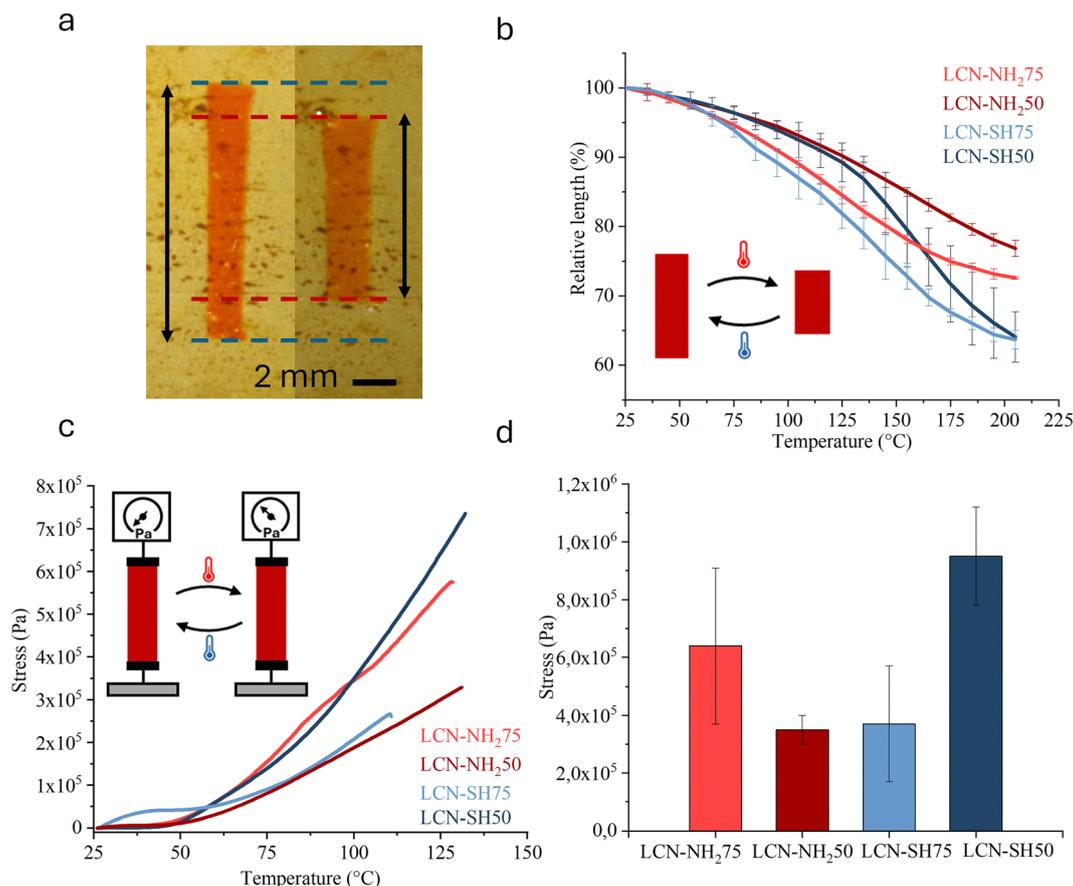
**Fig. 3 Thermal actuation of LCNs.** (a) Picture showing the thermal actuation under free standing conditions of an LCN-NH<sub>2</sub>75 sample at 25 °C (left) and 200 °C (right). (b) Thermal actuation under free standing conditions for all the LCN films. (c) Examples of one representative trace of tension vs. temperature for each LCN in thermal actuation experiments performed under isometric conditions. (d) Average over three measures of the maximum tension reached by each material.
