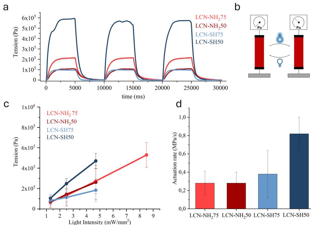
**Fig. 4 Photo-actuation of LCNs.** (a) Traces of tension developed by LCNs during light actuation at  $4.7 \text{ mW mm}^{-2}$ . (b) Schematization of light actuation experiment. (c) Average of the maximum tension developed by the materials vs. intensity of light. (d) Rate of actuation of LCNs at  $4.7 \text{ mW mm}^{-2}$ , obtained as the slope of the tangent in the first 200 ms of the tension traces.
