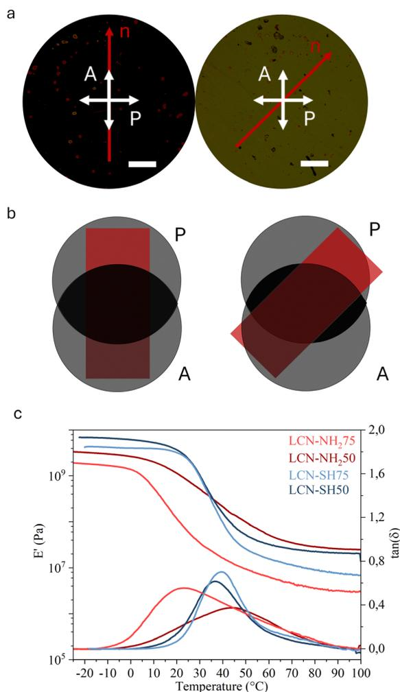
Fig. 2 Molecular alignment and mechanical tests on LCN films. (a) POM images of an LCN film with the director ( $n$ ) oriented orthogonally to the polarisers and at 45°. Scale bar: 200  $\mu\text{m}$ . (b) Schematization of the transmittance of LCN films under two crossed polarizer ( $P$ ) and analyser ( $A$ ). (c) Storage modulus ( $E'$ ) and  $\tan(\delta)$  representative curves for the LCNs synthesised.
