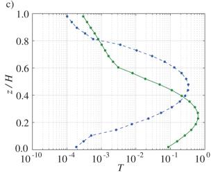
Fig. 7 Local time-averaged profiles of (a) solid volume fraction, (b) velocity in the flow direction and (c) granular temperature, for  $F_z$  = 24 000 with  $\mu_p$  = 0.01 (solid lines) and  $\mu_{\rm p}$  = 0.3 (dashed lines).
