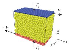
Fig. 1 A snapshot of the DEM simulation: the flowing particles (coloured in yellow) are sheared by moving the two planes in the opposite direction along the x-axis at a constant relative velocity of 2V.
