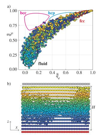
Fig. 5 (a) Time-averaged local order parameters for flowing particles of  $\mu_{\rm p}$  = 0.3 when  $F_{\rm z}$  = 2.4, coloured by their position in the z-direction. The sketched regions for bcc, hcp, fcc, and fluid phases are taken from Eslami et al. 33 (b) A snapshot of the particle positions projected on the x-z plane (particle size is scaled by 50% to facilitate the view)
