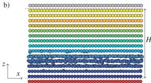
Fig. 8 (a) Time-averaged local order parameters for flowing particles of  $\mu_{\rm p}$  = 0.01 when  $F_{\rm z}$  = 24000, coloured by their position in the z-direction. The sketched regions for bcc, hcp, fcc, and fluid phases are taken from Eslami et al. 33 (b) A snapshot of the particle positions projected on the x-zplane (particle size is scaled by 50% to facilitate the view).
