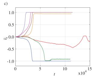
Fig. 2 Time evolution of (a) the average kinetic energy per particle, (b) the average volume fraction, (c) the velocity of the center of the mass of the flowing particles in the x-direction, for  $F_z = 2.4$  and different particle friction coefficients
