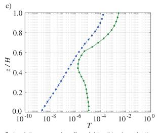
Fig. 3 Local time-averaged profiles of (a) solid volume fraction, (b) velocity in the flow direction and (c) granular temperature, for  $F_z$  = 2.4 with  $\mu_p = 0.01$  (solid lines) and  $\mu_p = 0.3$  (dashed lines).
