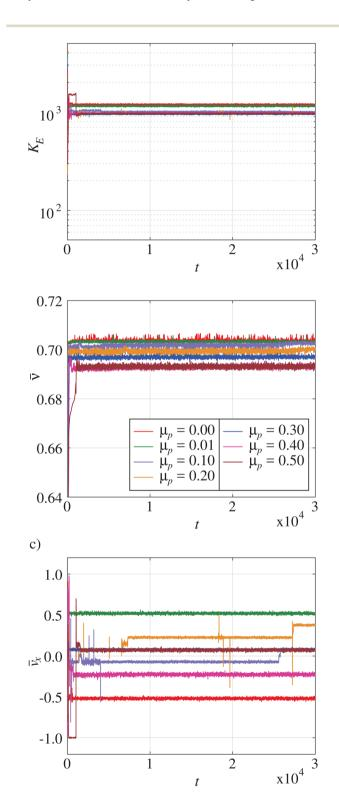
Fig. 6 Time evolution of (a) the average kinetic energy per particle, (b) the average volume fraction, (c) the velocity of the center of the mass of the flowing particles in the x-direction, for  $F_z = 24\,000$  and different particle friction coefficients.
