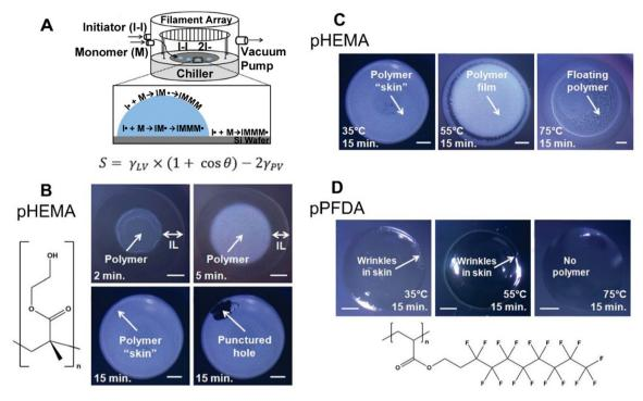
Fig. 4 (A) ILiCVD schematic with spreading coefficient expression. (B) pHEMA depositions on [bmim][PF<sub>6</sub>] with time as the variable changed. Scale bars are 1 mm. (C) Depositions with stage temperature as the variable changed. Scale bars are 1 mm. (D) pPFDA depositions on [bmim][PF<sub>6</sub>] for 15 minutes at different temperature conditions. Scale bars are 1 mm. Reprinted from ref. 66 with permission from American Chemical Society, Copyright 2011.
