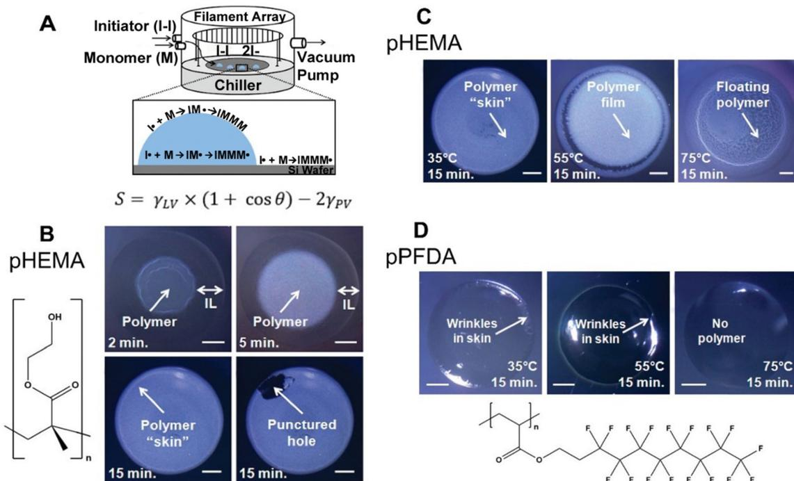
Fig. 4 (A) ILiCVD schematic with spreading coefficient expression. (B) pHEMA depositions on [bmim][PF<sub>6</sub>] with time as the variable changed. Scale bars are 1 mm. (C) Depositions with stage temperature as the variable changed. Scale bars are 1 mm. (D) pPFDA depositions on [bmim][PF<sub>6</sub>] for 15 minutes at different temperature conditions. Scale bars are 1 mm. Reprinted from ref. 66 with permission from American Chemical Society, Copyright 2011.
