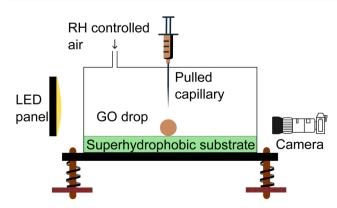
Fig. 1 Schematic of the experimental setup
