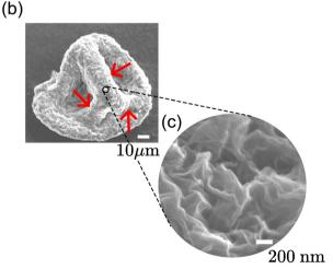
Fig. 2 (a) Time evolution of projected drop area A(t) for  $\phi_0 = 5.7 \times 10^{-5}$  and RH = 30%. The insets show the contours of drop edges (red curves) at selected times, superimposed on side view images of the drop. The black scale bars are 50  $\mu$ m. (b) SEM image of the buckled shell. (c) SEM image at higher magnification of the buckled shell surface shows nano-scale wrinkles.
