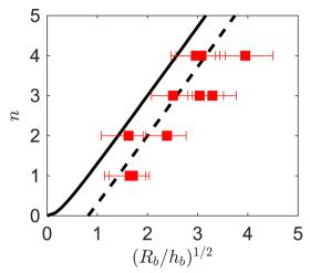
Fig. 10 Buckling mode number *n* vs.  $(R_{\rm b}/h_{\rm b})^{1/2}$  for  $\phi_0 \approx 5 \times 10^{-5}$ . The black curve corresponds to eqn (4). The black dashed line is n-1.
