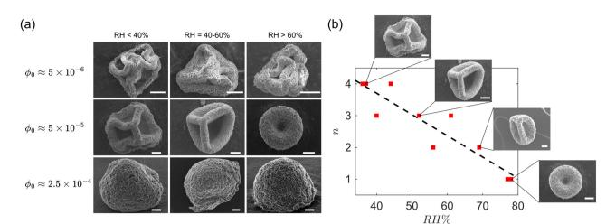
Fig. 9 (a) Scanning electron microscope (SEM) images of dried capsules for selected initial concentrations and relative humidity values. (b) Buckling mode number vs. relative humidity for  $\phi_0 \approx 5 \times 10^{-5}$ . Insets show corresponding SEM images of the buckled capsule. All the scale bars represent 20  $\mu$ m. Black dashed line serves as a visual guide. All experiments here correspond to GO drops with acidic pH.
