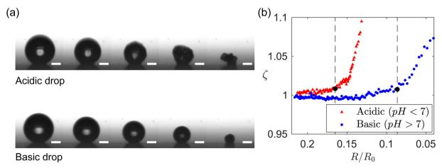
Fig. 6 (a) Time evolution of drop morphology comparing acidic and basic drops. The time increases in steps of 25 seconds. Scales bars represent 100  $\mu$ m. (b) Circularity parameter  $\zeta = P^2/(4\pi A)$  vs. normalized radius of the drop. Here P and A are the projected drop perimeter and area, respectively.
