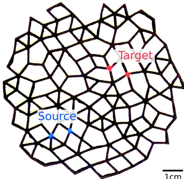
Fig. 1 Disordered elastic foam network labeled with source and target node pairs.
