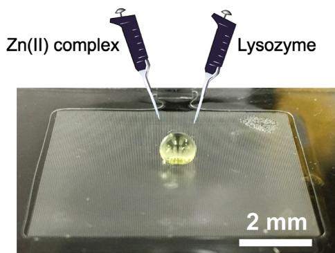
Fig. 6 Overview of crystallization experiment. Zn(II) complex and lysozyme were added dropwise and left for 120 min after the formation of the microdroplets.
