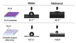
Fig. 8 Contact angles for the water-repellent device and an SU-8 substrate with water and methanol (n = 10).
