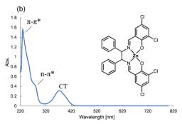
Fig. 10 Compound identification analysis. (a) IR spectrum. The peak near 1630 cm<sup>-1</sup> is due to C=N bonds. (b) UV-vis spectrum, containing a  $\pi - \pi^*$ transition at 225 nm, an  $n-\pi^*$  transition 285 nm, and a CT transition around 400 nm.
