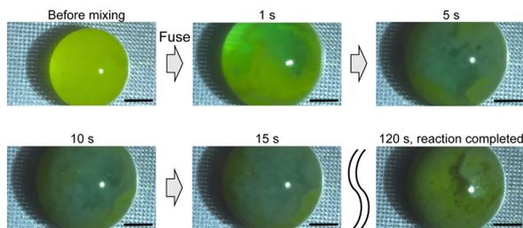
Fig. 9 Observation of the synthesis of a Zn(II) complex. 1 s: the chemical reaction begins as soon as the two reagents mix. 5 s: the metal complex begins to form. 10 s: microcrystals of the metal complex are dispersed in the droplet. 15 s: the reaction progresses as the microcrystals move within the droplet. 120 s: the movement of the microcrystals stops and the chemical reaction ends. Scale bar is 300 μm.
