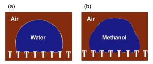
Simulation of droplet shape on an umbrella-shaped waterrepellent device. (a) Water microdroplet. (b) Methanol microdroplet.
