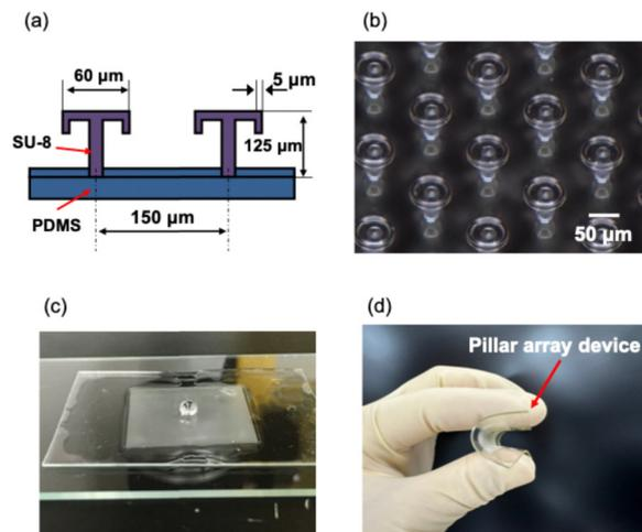
**Fig. 4** Dimensions and appearance of pillar array device. (a) Device dimensions. The umbrella diameter is 60 μm and the distance between pillars is 150 μm. (b) Micrograph of the umbrella-shaped pillars made of SU-8. (c) Photograph of a water drop on the umbrella-shaped pillar device. (d) Flexibility of pillar array devices.
