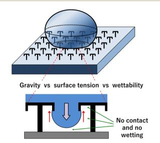
Fig. 1 Conceptual diagram of the pillar array device (top) and the principle of water repellence (bottom).
