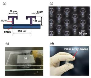
Dimensions and appearance of pillar array device. (a) Device dimensions. The umbrella diameter is 60 µm and the distance between pillars is 150  $\mu m$ . (b) Micrograph of the umbrella-shaped pillars made of SU-8. (c) Photograph of a water drop on the umbrella-shaped pillar device. (d) Flexibility of pillar array devices.
