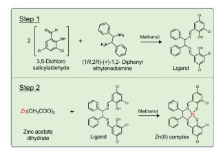
Fig. 5 Synthesis scheme of the Zn(II) complex. Step 1: Synthesis of the ligand from 3,5-dichlorosalicylaldehyde and (1R,2R)-(+)-1,2-diphenylethylene-diamine. Step 2: Synthesis of the Zn(II) complex from the ligand and zinc acetate
