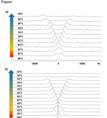
Fig. 7 Stackplot of <sup>2</sup>H NMR spectra recorded on cooling the sample from the isotropic phase to the crystal phase for the samples (a) 3F5HPhF9 with a small amount of biphenyl-4,4 $^{\prime}$ -diol-d<sub>4</sub> and (b) 3F7HPhF8 with a small amount of biphenyl-4,4'-diol-d4.
