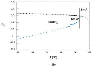
Fig. 11 (a) Experimental orientational order parameter  $S_{zz}^{\exp}(T)$  determined by NMR with  $\varDelta_{\rm biax}=0$  (orange symbols) and (b) experimental orientational order parameter  $S_{zz}^{\exp}(T)$  determined by NMR with  $\varDelta_{\rm biax}=0.05$  (blue symbols) superimposed with the values (black symbols) of the mesophase orientational order  $S_{zz}^n(T)$  extrapolated from the SmA phase of the 3F7HPhF8 sample. The black curve is the best fitting curve by using eqn (4).
