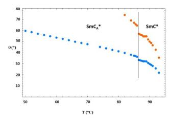
Fig. 12 Values of the tilt angle  $\theta(T)$  obtained by using eqn (3) as described in the text. The blue symbols refer to the case of  $\Delta_{\rm biax}$  = 0.05 and the orange symbols refer to the case of  $\Delta_{\text{biax}}$  = 0.
