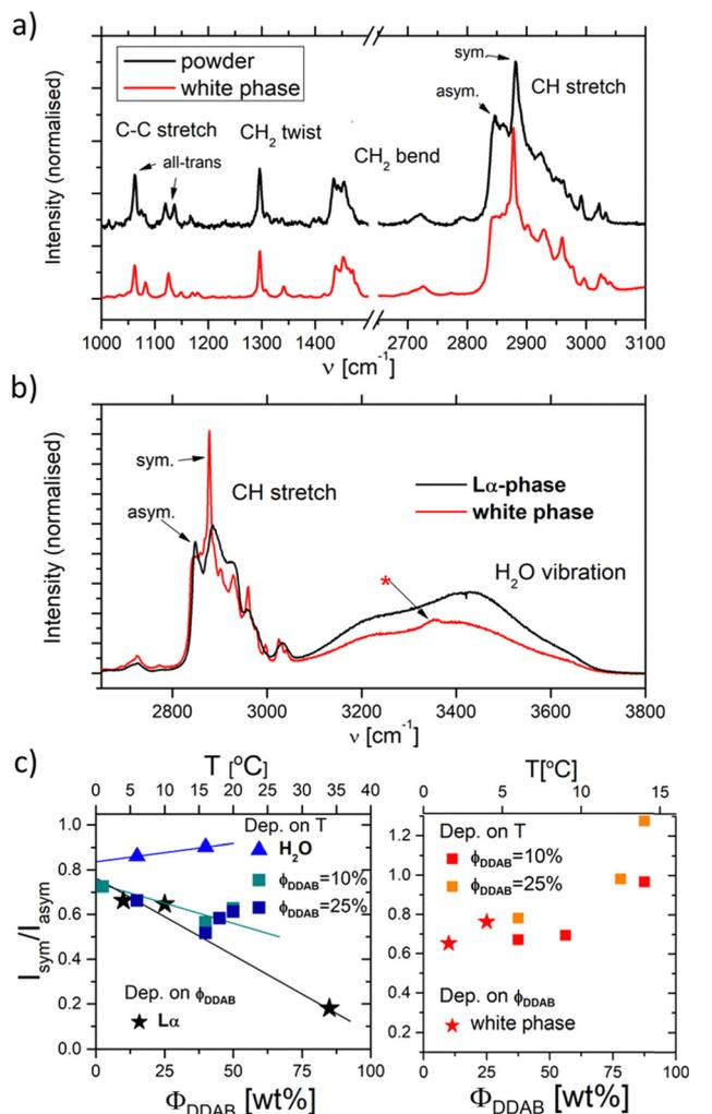
Fig. 6 (a) and (b) Raman spectra of aqueous DDAB solution in the lamellar phase (black) compared to the 'white' phase (red). (c) Ratio of the  $I_{\text{sym}}/I_{\text{asym}}$  water peaks depending on DDAB concentration, phase and temperature (see also the ESI,† Table S1).
