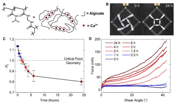
Fig. 5 (A) Chemical structures of NIPAM and calcium crosslinked alginate used to fabricate the hydrogel interior. (B) Photographs of hydrogel/LEGO hybrid unit cell at room temperature swelling equilibrium (left), and after 24 hours of immersion in 34 °C DI water (right). (C) Linear swelling ratio of NIPAM/alginate gels as a function of time immersed in 34 °C DI water. (D) Force vs. shear angle for hydrogel/LEGO hybrid unit cells taken at several different times of immersion in 34 °C DI water.
