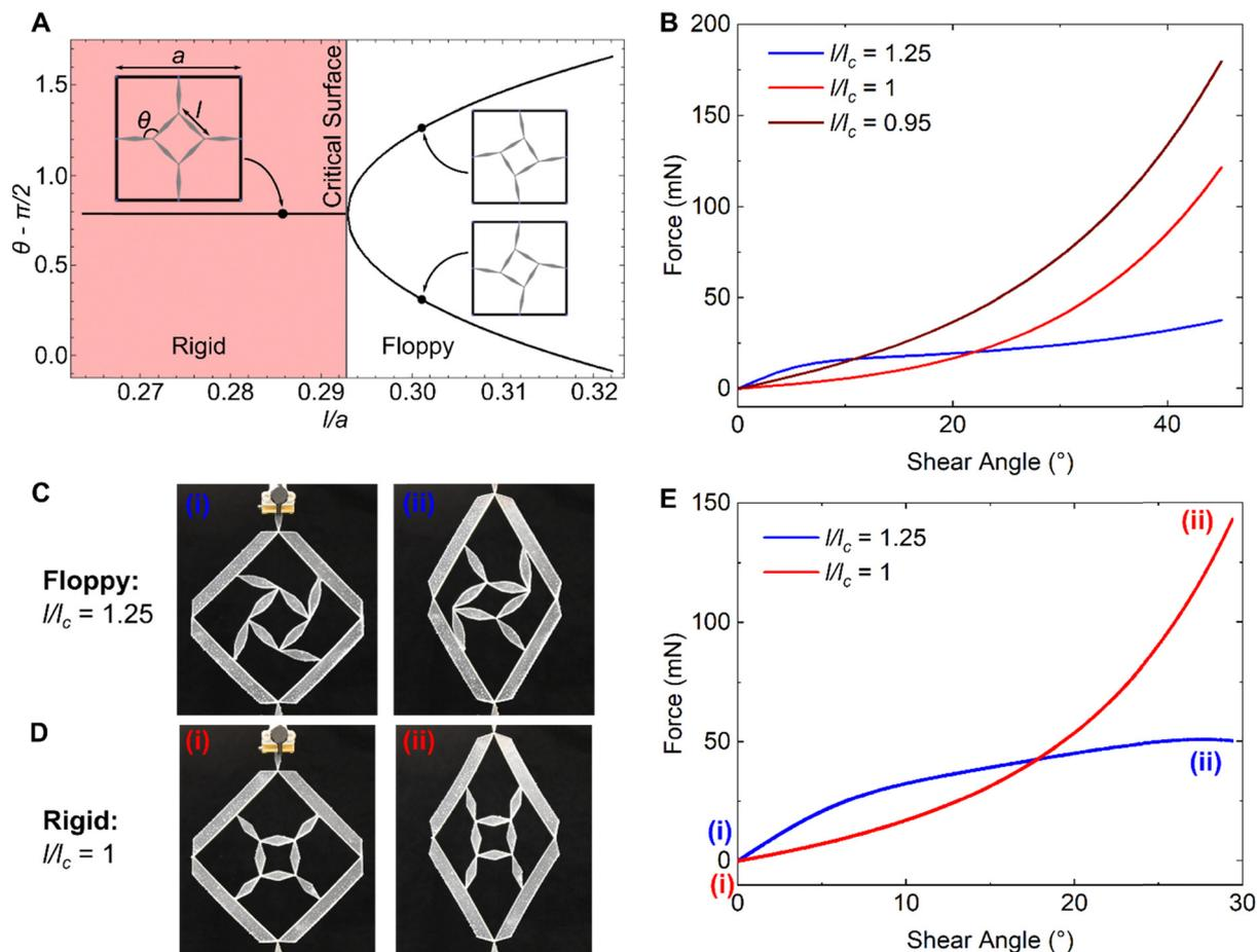
**Fig. 1** (A) Phase diagram for the 2nd order rigid unit cell depicted in the insets. (B) Calculated force vs. shear response of the unit cell. (C) Photographs of a 3D printed floppy unit cell at (i) zero shear and (ii)  $30^\circ$  shear angle. (D) Photographs of the unit cell with beams shrunk to the critical point at (i)  $0^\circ$  and (ii)  $30^\circ$  shear angle. (E) Force vs. shear angle response for rigid and floppy structures.
