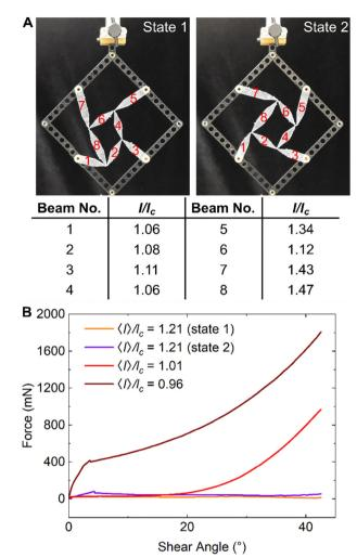
Fig. 4 (A) Photographs of LEGO/3D printed unit cells with randomly generated beams lengths in state 1 (left) and state 2 (right). The beams are numbered on the image and the randomly generated  $l/l_c$  values are given in the table below. (B) Force vs. shear angle for randomly generated LEGO/3D printed unit cells.
