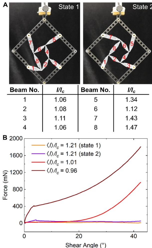
Fig. 4 (A) Photographs of LEGO/3D printed unit cells with randomly generated beams lengths in state 1 (left) and state 2 (right). The beams are numbered on the image and the randomly generated  $l/l_c$  values are given in the table below. (B) Force vs. shear angle for randomly generated LEGO/3D printed unit cells.
