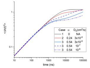
Fig. 10 Long time calculations of  $\langle \Delta h^2(t) \rangle$  for cases 1–3 with different values of  $D_0$  for case 3.
