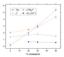
Fig. 9 Results that include dynamical diffusional softening theory in fits that constrained  $\eta_{\rm m}$  to its value with no cholesterol. The obtained values of  $\alpha$  (times 10, upward triangles) were used to fit the data resulting in the membrane viscosity (circles) and the unsoftened  $\kappa$  obtained from eqn (10).
