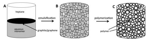
Scheme 1 Schematic describing the preparation of the conductive hydrogel. (A) Heptane, graphite, and aqueous monomer are placed in a flask. (B) Emulsifying the mixture results in aqueous drops, which are stabilized by a thin layer of overlapping graphene sheets and suspended in a continuous oil phase. (C) Subsequent monomer polymerization results in a porous, electrically conductive hydrogel after removing the oil phase by evaporation.
