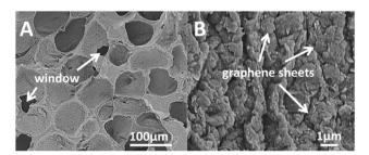
Fig. 3 Scanning electron micrograph of (A) a cross-section of a dried hydrogle composite showing windows connecting the cells of the foam. (B) Higher magnification image illustrating the graphene present on the inner walls of the foam cells.
