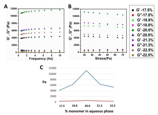
Fig. 6 Rheological behavior of hydrogels. (A) G' and G" vs. frequency for hydrogels made with different monomer concentrations. (B) G' and G" values at constant frequency (1 Hz) for hydrogels made with different monomer concentrations. (C) Comparison of G' and G'' as a function of monomer concentration, where the upper blue line is G' and lower red line is G''. Values of G' are averaged values obtained from the frequency sweep shown in (A).
