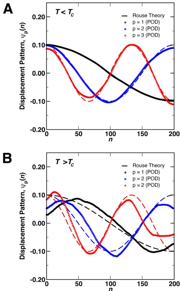
Fig. 2 Displacement patterns (*i.e.*, eigenfunctions) of the first three relaxation modes of a single, free polymer chain ( $N = 200$ ) determined from proper orthogonal decomposition (POD, points) compared to the analytical result from the Rouse Model (dashed lines) for (A)  $T < T_c$  and (B)  $T > T_c$ .
