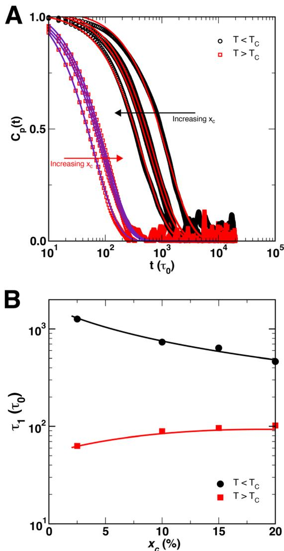
Fig. 7 (A) Temporal autocorrelation function  $C_p(t)$  ( $\rho = 1$ ) for SCNPs ( $N = 200$ ) as a function of  $x_c$  for  $T < T_c$  (black circles) and  $T > T_c$  (red squares). The lines are fits to eqn (12) with  $\beta = 1$ . The arrows denote the variation of  $x_c$ . (B) Relaxation times of the first mode, obtained from the data in (A), as a function of  $x_c$ , plotted for SCNPs below  $T_c$  (black circles) and above  $T_c$  (red squares). The lines are guides for the reader.
