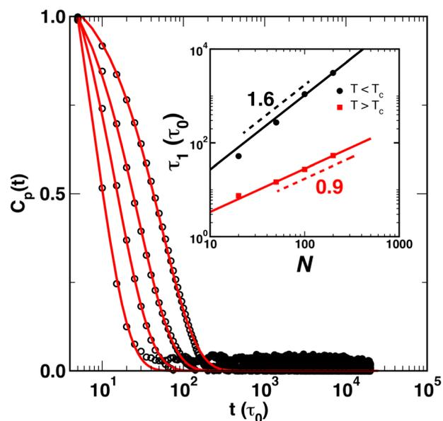
Fig. 4 Normal mode temporal autocorrelation function  $C_p(t)$  plotted for the lowest mode  $p = 1$  as a function of time above  $T_c$ . Red curves are fits to eqn (12) with  $\beta = 1$  for (left to right)  $N = 20, 50, 100$ , and 200. The inset presents the scaling of the longest relaxation time  $\tau_1$  with degree of polymerization  $N$ . The dashed curves correspond to the scaling exponent for  $T < T_c$  (black) and  $T > T_c$  (red).
