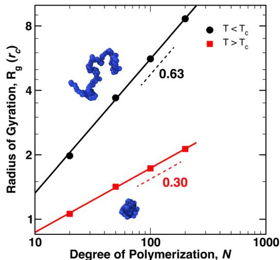
Fig. 1 Average radius of gyration,  $R_g$ , plotted as a function of degree of polymerization,  $N$ . Circles correspond to coil conformations below  $T_c$  while squares correspond to globular conformations above  $T_c$ . The rendered polymers depict representative coil (top) and globule (bottom) conformations for  $N = 100$ . Error bars, corresponding to one standard deviation in the value of  $R_g$  are smaller than the size of the points.
