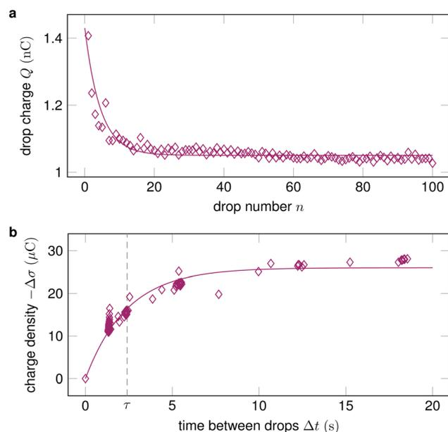
Fig. 3 (a) The drop charge at a fixed position  $x$  along the slide path decreases and then saturates with increasing drop number. Data reproduced from ref. 19; (b) By varying the time between drops  $\Delta t$  and measuring the change in surface charge density  $\Delta\sigma$ , the characteristic discharge time  $\tau$  can be quantified. Data reproduced from ref. 32.
