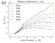
Fig. 9 Values of diffusion coefficients from MD simulations. (a) Diffusion constants at T = 387 K as a function of lattice constant. The vertical lines are the lattice constants at the two solvent concentrations. (b) Diffusion coefficient for different temperatures for  $\Phi_{\rm v} \approx 0.18$ . (c) Diffusion coefficient for different temperatures for  $\Phi_{\rm v} \approx 0.3$ .
