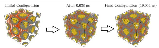
Fig. 1 Summary of a typical simulation: a bcc configuration with  $a_L = 63 \text{ Å}$  and  $\Phi_v = 0.18$ . The solvent (hexane) is marked in red. In the left there is the initial configuration, which after only 0.381 ns is roughly thermalized. The configuration at the end of the simulation (19.064 ns) is shown.
