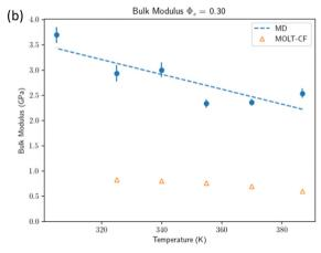
Fig. 4 Comparison of bulk modulus eqn (16) MOLT-CF vs. MD simulations. See the ESI† for additional plots and a more elaborated discussion. (a) Bulk modulus for the dry system. (b) Bulk modulus for the swollen system.
