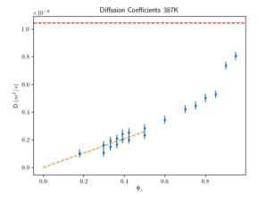
Fig. 10 Hexane diffusion coefficient from MD simulations as a function of  $\Phi_{\rm v}$  at the minimum of the free energy for T=387. The dashed red line is the diffusion coefficient for hexane. The dashed orange fit shows that the limit of the diffusion at a low volume fraction is consistent with zero
