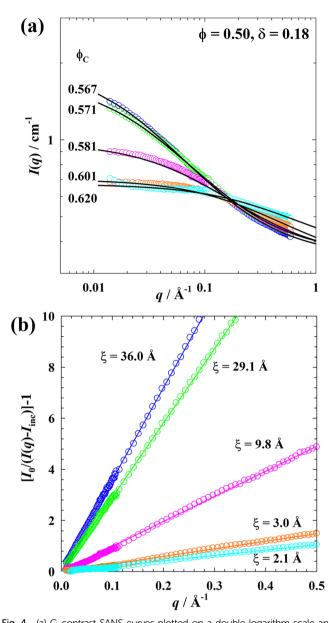
Fig. 4 (a) C-contrast SANS curves plotted on a double logarithm scale and (b)  $[I_0/(I(q) - I_{inc})] - 1$  plotted versus q for the quasi-ternary system D<sub>2</sub>Ocyclohexane-D<sub>12</sub>/cyclohexane (85/15)-2-propanol-OD/1-propanol-OD measured as a function of the total alcohol volume fraction  $\phi_{\rm C}$  at  $\delta$  = 0.18,  $\phi$  = 0.50, and T = 25.0 °C.  $\xi$ -Values were obtained from the slope of the plot.
