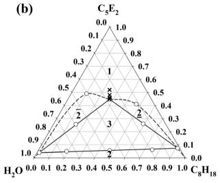
Fig. 7 Gibbs triangles (volume fraction) of the ternary systems (a)  $H_2O-n$ octane $-C_4E_1$  measured at T = 19.5 °C and (b)  $H_2O-n$ -octane $-C_5E_2$  measured at T = 33.7 °C. Black crosses illustrate the SANS study measured as a function of  $\phi_{\rm C}$  in bulk-contrast at equal volumes of water and oil, i.e.,  $\phi = 0.50$ .
