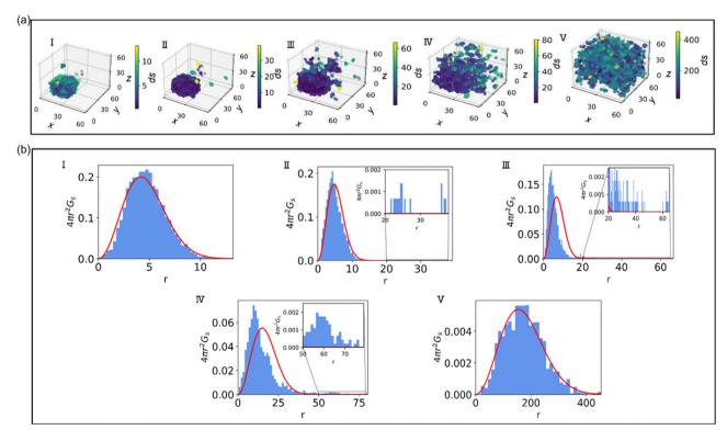
Fig. 3 (a) Heat map of displacements (ds) of reactive beads during the degradation of nanogel at the time instants marked (I-V) in Fig. 2. (b) Probability density of the displacements of reactive beads at the same time instants; bar plots in blue represent simulation data, and red curves represent Gaussian distribution. The insets in (II-IV) show close-up of the probability density at higher distances as marked.
