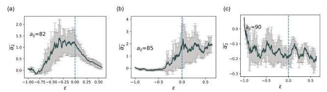
Fig. 8 Non-Gaussian parameter,  $\alpha_2$ , as a function of the relative extent of reaction,  $\epsilon$ , of reactive beads for cases B, C and D in (a)–(c), respectively. Averages are taken over five independent degradation simulation runs
