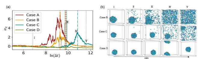
Fig. 6 (a) Time evolution of the non-Gaussian parameter during the degradation process for cases A, B, C, and D as marked in the legends. A single simulation (seed r1) is shown for each parameter set. (b) Simulation snapshots at time instants marked (I–V) in (a) for cases B, C, and D in top, bottom, and middle row, respectively. Water beads are not shown for clarity of representation.
