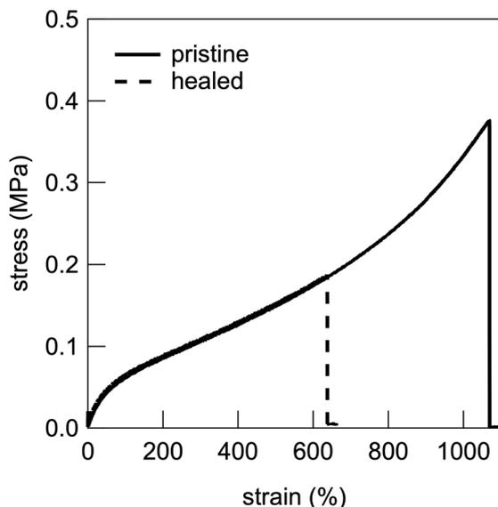
Fig. 6 Stress–strain curves of pristine and healed PMMA-LiFSI-PEGDME UHMW gel samples.
