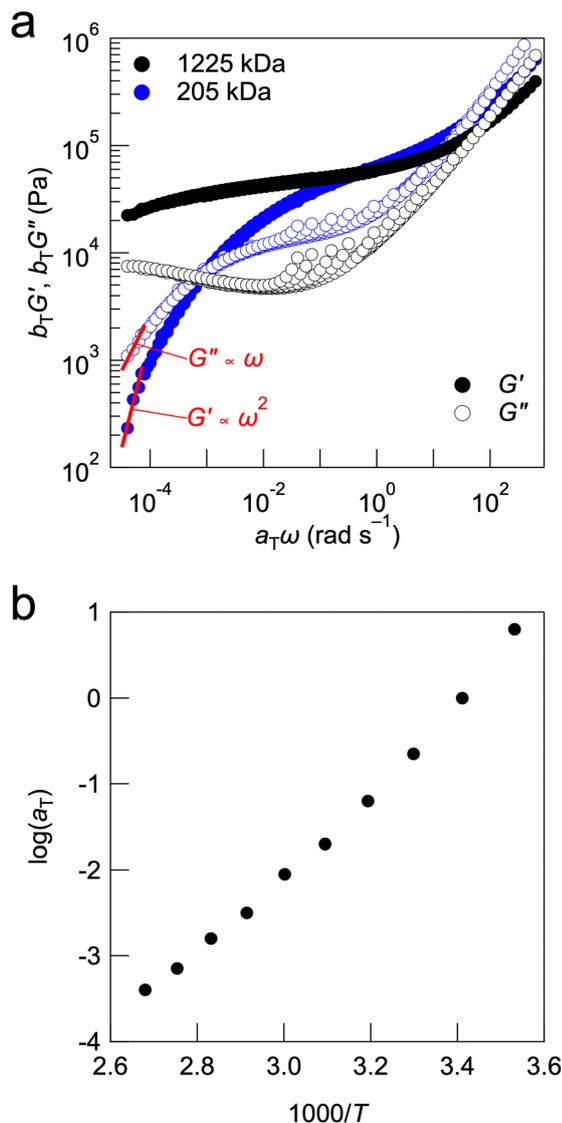
Fig. 4 (a) tTS master curves for PMMA-LiFSI-TEGDME composites with moderate molecular weight and UHMW PMMA. The reference temperature is 20 °C. (b) Arrhenius plot of the shift factor ( $a_T$ ) for both PMMA-LiFSI-TEGDME systems.
