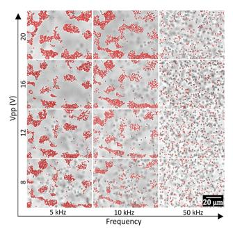
Fig. 3 Peak to peak voltage  $(V_{pp})$  versus frequency optical micrograph of 1 µm polystyrene spheres functionalised with amine ( $\zeta = -94.6$  mV) Cluster size increases with voltage at intermediate frequencies, with no significant effect at low and high frequencies.
