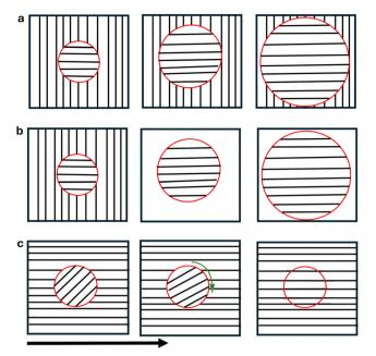
Fig. 1 Different mechanisms of alignment of a lamellar system: (a) nucleation and growth of stable domains or shrinking of the unstable ones: (b) partial melting of the unstable domains: (c) rotation of the unstable domains The arrow indicates the direction of the applied external field
