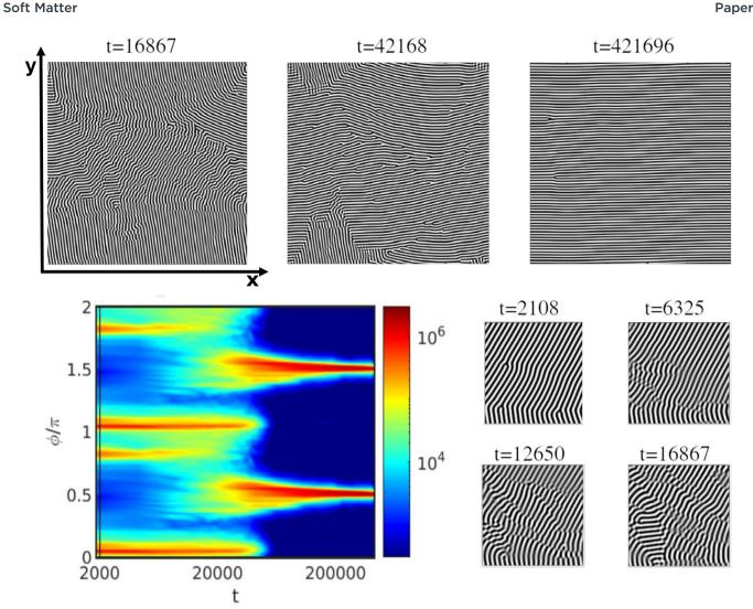
Fig. 11 Rotation in 2D with  $\tau = 0.29$  and  $L_z/H_0 = 1$  under a shear flow rate  $\dot{\gamma} = 0.0024$  (Wi =  $1.4 \times 10^{-2}$ ). The colourmap of the scattering intensity  $S(\phi)$  is shown along with snapshots of the x-y plane  $z=L_z/2$  with time shown above each snapshot.
