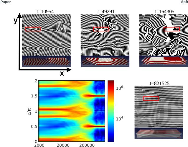
Fig. 12 Rotation 3D for a system under a shear rate  $\dot{\gamma} = 0.00183$  and  $\tau = 0.36$  for a thicker film with  $L_z/H_0 = 2$  (Wi =  $7.1 \times 10^{-3}$ ). The colourmap of the scattering intensity  $S(\phi)$  is shown along with snapshots of the two-dimensional x-y plane at  $z=L_z/2$  with time shown above each snapshot. The respective top-view 3D images show a subset of the full system box.
