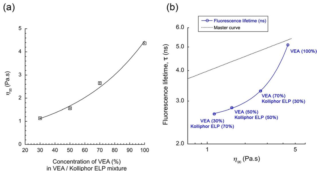
Fig. 7 Characterization of the mixture VEA/Kolliphor ELP (nonionic surfactant). (a) Viscosity for different compositions, and (b)  $\tau$  of rBDP-Toco as a function of the viscosity, in these VEA/Kolliphor ELP mixtures (where the composition is indicated as labels in the graph). The comparison with the master curve obtained with oil mixtures is also reported in the figure.
