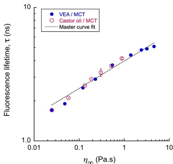
Fig. 3 Fluorescence lifetime ( $\lambda_{\text{ex}} = 460$  nm,  $\lambda_{\text{em}} = 512$  nm) of rBDP-Toco dissolved in different oil mixtures, represented against viscosities of oil mixtures of VEA or castor oil concentration (%) mixed with MCT.
