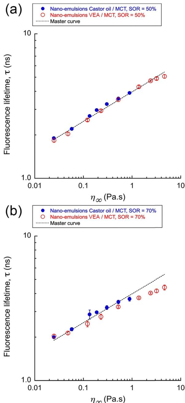
Fig. 5  $\tau$  of nano-emulsions made with different oil mixtures (detailed in the legend), as a function of the viscosities ( $\eta_{\infty}$ ) of the corresponding oil mixtures composing their core (from Fig. 1). (a) SOR = 50% and (b) SOR = 70%.
