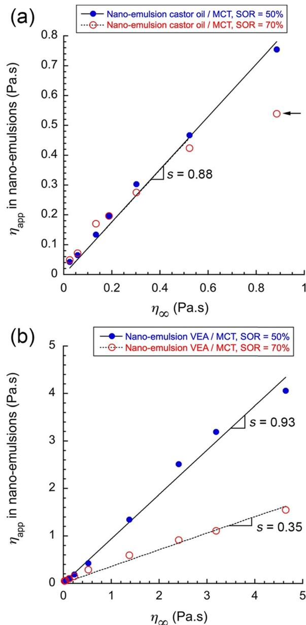
Fig. 6 Comparison of viscosities between oil mixture in the core of nano-emulsion droplets ( $\eta_{app}$ ) and pure oil mixtures ( $\eta_{\infty}$ ), for two different SOR (SOR = 50% and 70%), and for two different compositions of oil mixtures: castor oil/MCT (a), and VEA/MCT (b). Linear extrapolation and related slopes ( $s$ ) are indicated in the figures (excluding nano-emulsions formulated with pure castor (arrow in a)).
