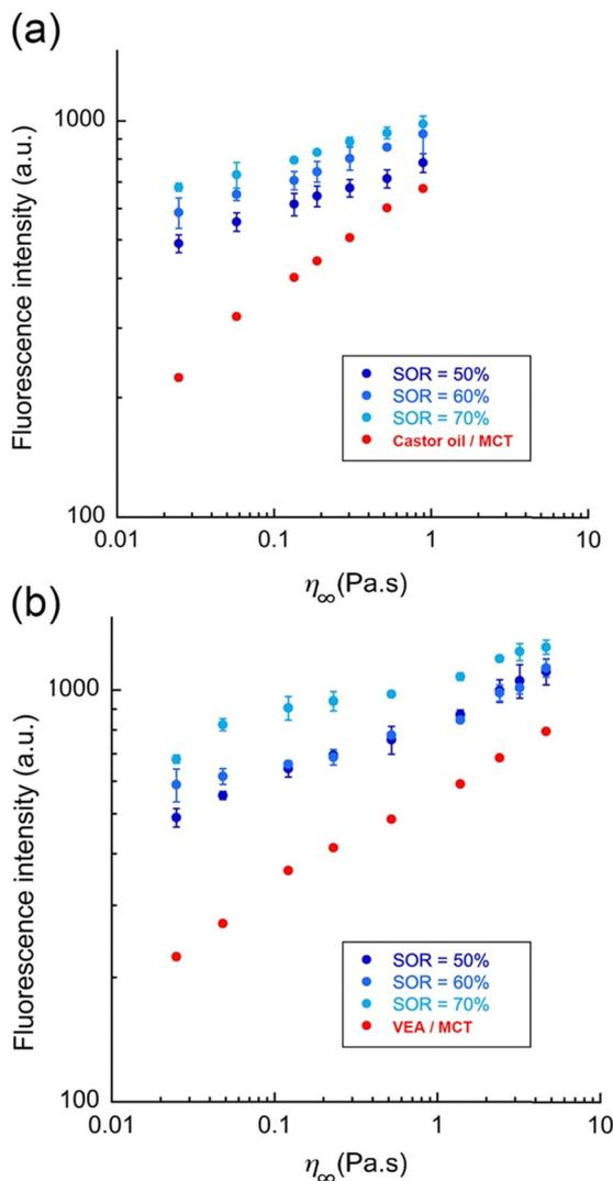
Fig. 8 FI of oil mixtures and their respective nano-emulsions formulations in function of the viscosities ( $\eta_{\infty}$ ) of the different oil mixtures: (a) castor oil/MCT and (b) VEA/MCT. Different nano-emulsion size range was compared to each other and compared with pure oil mixture. FI intensity was normalized to the oil amounts in the formulations.
