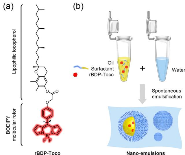
**Scheme 1** (a) Structure of rBDP-Toco. The viscosity fluorescent reporter is a BODIPY molecular rotor, the lipophilicity was enhanced by coupling with the lipid tocopherol. (b) Principle of the nano-emulsion formulation by spontaneous emulsification.
