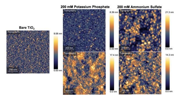
Fig. 5 AFM height images of silk fibroin coatings formed in potassium phosphate (middle top), ammonium sulfate (right top), acetic acid buffer (middle bottom), and potassium sulfate (bottom right). Potassium phosphate promotes smooth, uniform globular surface topography. All other kosmotropic salts form coatings with exposed underlying substrate (TiO2, left) and are not as uniform
