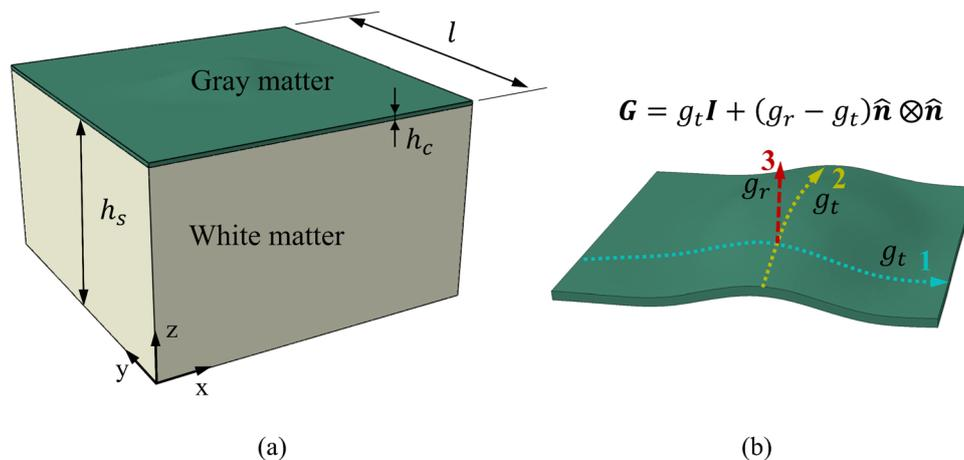
Fig. 4 Geometric model for modeling regional brain growth. (a) Initial status of a FEM model,  $h_c$  and  $h_s$  represent the layer thickness of gray matter and white matter, respectively; (b) orthogonal growth patterns,  $g_t$  and  $g_r$  indicate the tangential growth ratio within the plane and radial growth ratio in the thickness direction, respectively.
