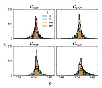
Fig. 5 Histograms of rigidity percolation threshold  $p_c$  as a function of system size L at isotropy. The estimated density functions for each independent elastic modulus are plotted. Each distribution becomes increasingly sharp with larger system size.
