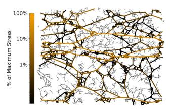
Fig. 4 Generic, isotropic triangular lattice strained in the horizontal direction until it becomes rigid, forming straight lines of bonds important for rigidity. The bonds are shaded corresponding to the energy contributed. Preliminary results suggest that one of the four tangent moduli  $(C_{xyxy})$ remains zero for a range of strains above the strain stiffening threshold, with  $C_{xxxx}$  being the dominant modulus.
