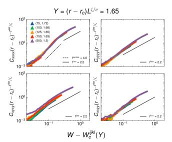
Fig. 18 Estimate of anisotropic scaling exponent of each modulus at a constant Y = 1.65. The simulation data is the same as found in Fig. 16
