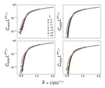
Fig. 10 Universal scaling function of all independent elastic modulus using previously reported exponents.<sup>6</sup> The data for the range  $L \in$ [30,200] comparable to the earlier work does give a good collapse. Having the larger system size (L = 500) explains why we find different exponents.
