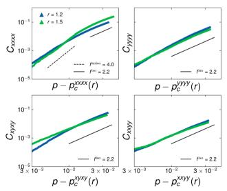
Fig. 14 Estimate of anisotropic scaling exponent of each modulus from our largest system size. The behavior of the  $C_{xxxx}$  modulus suggests a crossover between the anisotropic and isotropic scaling exponents, whereas for the other moduli, the behavior appears to be governed by the same isotropic exponent.
