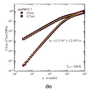
Fig. 6 Storage,  $G'(\omega)$ , and loss moduli,  $G''(\omega)$ , as a function of frequency,  $\omega$ , for (a) linear PBO and (b) star PBO at the reference temperature,  $T_{\text{ref}} = 248 \text{ K}$ . Solid lines are the best description of the Rouse model, eqn (6) and (7).
