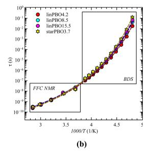
Fig. 10 (a) Susceptibility,  $\chi''(\omega \cdot \tau)$ , as a function of normalized frequency,  $\omega \cdot \tau$ , for all linear PBO samples as indicated at the reference temperature,  $T_{\rm ref} =$ 250 K. (b) Relaxation times,  $\tau$ , as a function of 1000/T for four selected samples as a combination of dielectric and FFC NMR data. Dashed lines are the best description of the VFT function.
