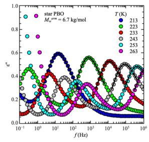
Fig. 1 Imaginary part of the permittivity,  $\varepsilon''$ , as a function of frequency, f, for one selected starPBO6.7 with  $M_{\rm w}^{\rm arm}$  = 6.7 kg mol<sup>-1</sup> as an example. Solid lines are the best description of the relaxation peak with the Havriliak-Negami function. Data points at very low frequencies are the conductivity contribution, which is not included in further discussions.
