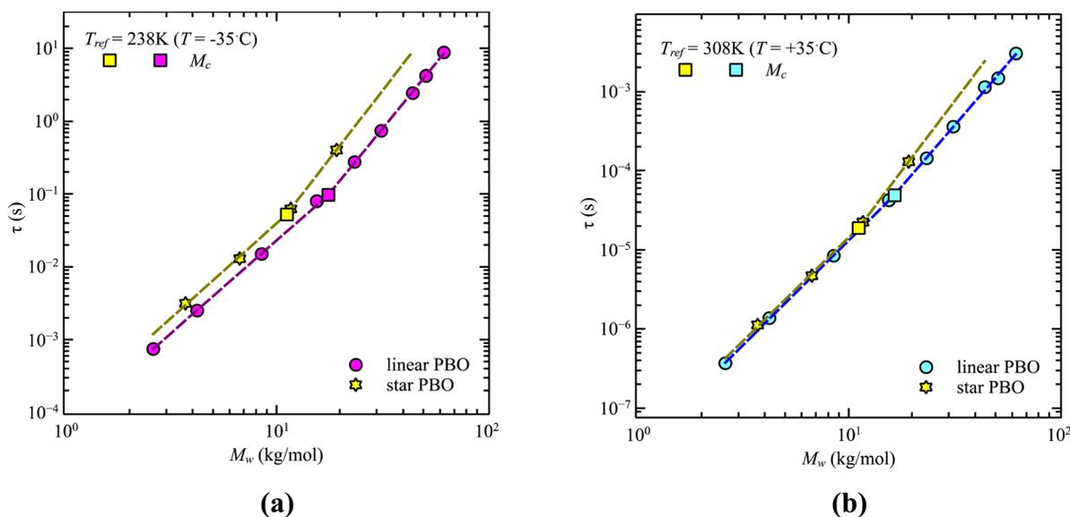
Fig. 4 Relaxation time,  $\tau$ , as a function of weight average molecular weight,  $M_w$ , for the comparison of linear PBO and star PBO at (a)  $T = 238$  K and (b)  $T = 308$  K. Dashed lines are the power law descriptions. The critical molecular weight is indicated by square symbols. Due to synthesis reasons, for the star polymer, only two molecular weights were available for each section.
