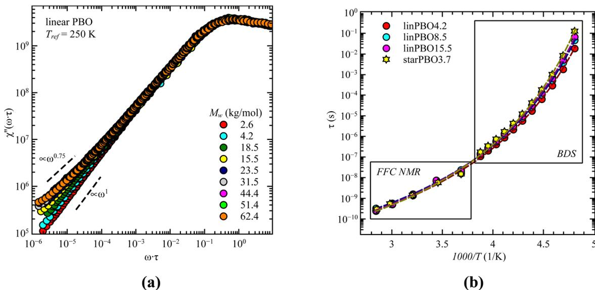
Fig. 10 (a) Susceptibility,  $\chi''(\omega\tau)$ , as a function of normalized frequency,  $\omega\tau$ , for all linear PBO samples as indicated at the reference temperature,  $T_{ref} = 250$  K. (b) Relaxation times,  $\tau$ , as a function of  $1000/T$  for four selected samples as a combination of dielectric and FFC NMR data. Dashed lines are the best description of the VFT function.
