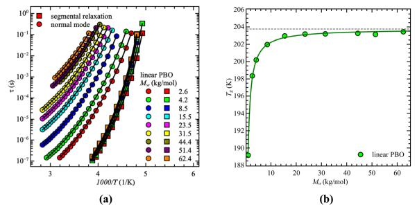
Fig. 2 (a) Relaxation time,  $\tau$ , as a function of 1000/T for the linear PBO samples. Solid lines are the best description of the VFT equation. (b) glass transition temperature, T<sub>o</sub>, as a function of molecular weight for the linear PBO samples. The solid line is the best description of the Fox-Loshaek law.
