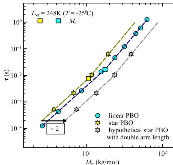
Fig. 8 Relaxation time,  $\tau$ , as a function of weight averaged molecular weight,  $M_w$ , for linear PBO and star PBO from the dielectric spectroscopy experiment. Grey data points are the relaxation times of the hypothetical star polymers having double the arm length, according to the rheology findings.
