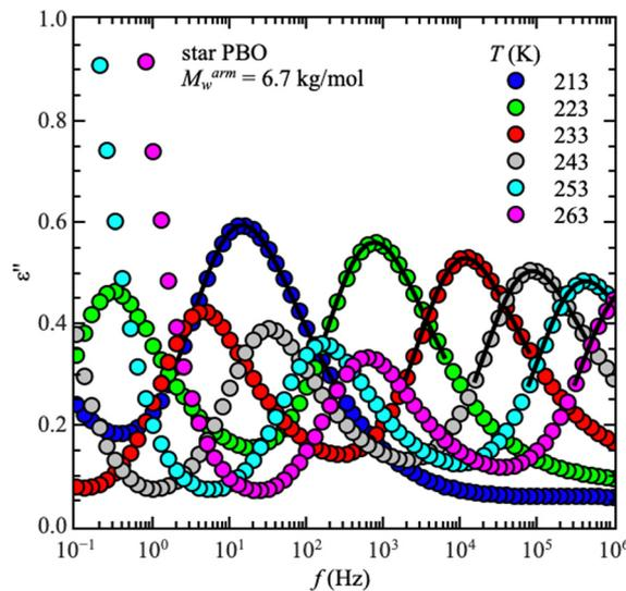
Fig. 1 Imaginary part of the permittivity,  $\epsilon''$ , as a function of frequency,  $f$ , for one selected starPBO6.7 with  $M_w^{\text{arm}} = 6.7 \text{ kg mol}^{-1}$  as an example. Solid lines are the best description of the relaxation peak with the Havriliak–Negami function. Data points at very low frequencies are the conductivity contribution, which is not included in further discussions.
