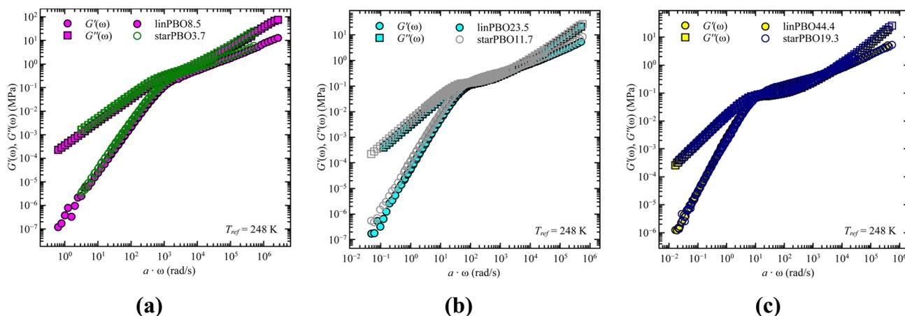
Fig. 7 Storage,  $G'(\omega)$ , and loss moduli,  $G''(\omega)$ , as a function of frequency,  $\omega$ , for the comparison of linear (filled symbols) and star PBO (open symbols) for (a) linPBO8.5 *vs.* starPBO3.7, (b) linPBO23.5 *vs.* starPBO11.7, and (c) linPBO44.4 *vs.* starPBO19.3.
