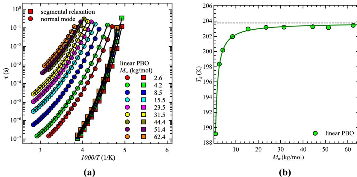
Fig. 2 (a) Relaxation time,  $\tau$ , as a function of  $1000/T$  for the linear PBO samples. Solid lines are the best description of the VFT equation. (b) glass transition temperature,  $T_g$ , as a function of molecular weight for the linear PBO samples. The solid line is the best description of the Fox–Loshak law.
