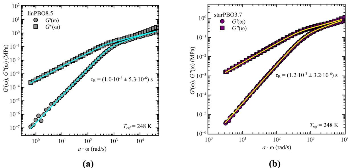
Fig. 6 Storage,  $G'(\omega)$ , and loss moduli,  $G''(\omega)$ , as a function of frequency,  $\omega$ , for (a) linear PBO and (b) star PBO at the reference temperature,  $T_{ref} = 248$  K. Solid lines are the best description of the Rouse model, eqn (6) and (7).
