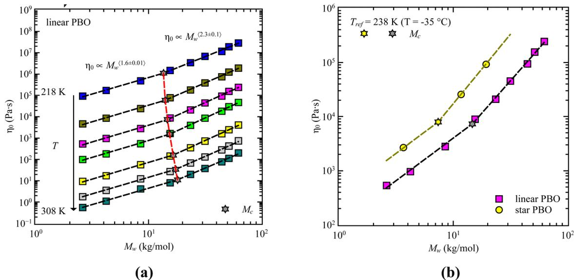
Fig. 9 Zero shear viscosity,  $\eta_0$ , as a function of weight averaged molecular weight,  $M_w$ , for (a) all the linear PBO samples at different temperatures, and (b) for the comparison between star PBO and linear PBO. Dashed lines are the best description of power laws.
