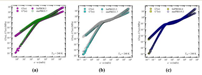
Fig. 7 Storage,  $G'(\omega)$ , and loss moduli,  $G''(\omega)$ , as a function of frequency,  $\omega$ , for the comparison of linear (filled symbols) and star PBO (open symbols) for (a) linPBO8.5 vs. starPBO3.7, (b) linPBO23.5 vs. starPBO11.7, and (c) linPBO44.4 vs. starPBO19.3.
