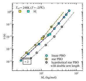
Fig. 8 Relaxation time,  $\tau$ , as a function of weight averaged molecular weight,  $M_{w_i}$ , for linear PBO and star PBO from the dielectric spectroscopy experiment. Grey data points are the relaxation times of the hypothetical star polymers having double the arm length, according to the rheology findings.
