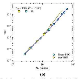
Fig. 4 Relaxation time,  $\tau$ , as a function of weight average molecular weight,  $M_{wv}$  for the comparison of linear PBO and star PBO at (a) T=238 K and (b) T = 308 K. Dashed lines are the power law descriptions. The critical molecular weight is indicated by square symbols. Due to synthesis reasons, for the star polymer, only two molecular weights were available for each section.
