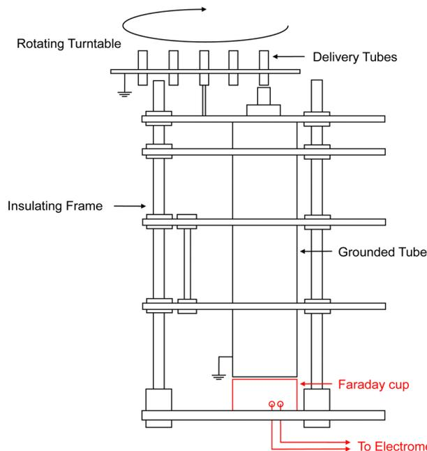
Fig. 2 A schematic of the ash charge apparatus for this work, adapted from Houghton *et al.* with the Faraday cup highlighted in red.<sup>1</sup>
