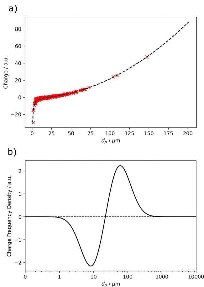
**Fig. 6** (a) The EDMD simulated charging against size ( $d_p$ ) for a monomodal fit of a sample of ash from Mount St. Helens where the charge carriers are negative and have arbitrary units of 1. The fit, shown as a dashed line, is a polynomial of the form  $f(d_p) = ad_p^2 + cd_p^{-1}$ , where  $a = 0.00218$  and  $c = -23.7$ . (b) The convolution of the charging and size distributions to give a charge frequency density distribution.
