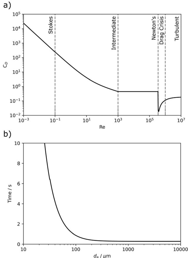
Fig. 5 (a) The dependency of the drag coefficient ( $C_D$ ) on the Reynolds number (Re) with the drag regimes labelled. (b) The predicted time for spherical particles to reach the Faraday cup (drop 37.25 cm) as a function of their aerodynamic diameter ( $d_a$ ).
