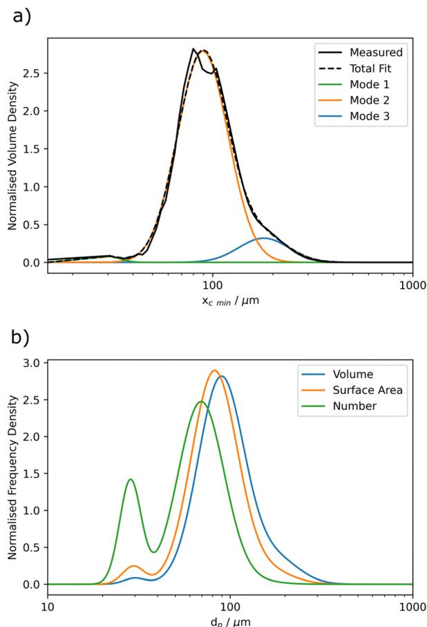
Fig. 4 (a) The trimodal fit for a volumetric size distribution was experimentally obtained using a CAMSIZER X2<sup>®</sup> on a sample of ash from the Atitlán volcano. (b) The volume distribution is converted using a spherical particle approximation to the surface area and number distributions.
