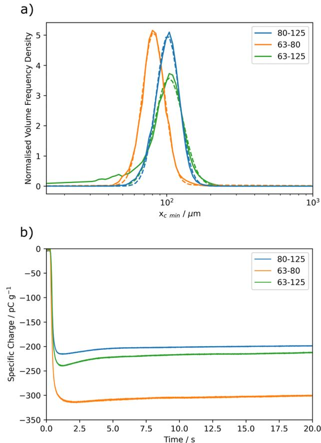
Fig. 8 (a) The volumetric size distributions for sieved fractions of Grímsvötn ash, obtained using a CAMSIZER X2<sup>®</sup> and fit with monomodal log-normal distributions. The ranges in the legend of the sieved fractions have the units of microns. (b) The Faraday cup traces for the corresponding sieved fractions of Grímsvötn ash.
