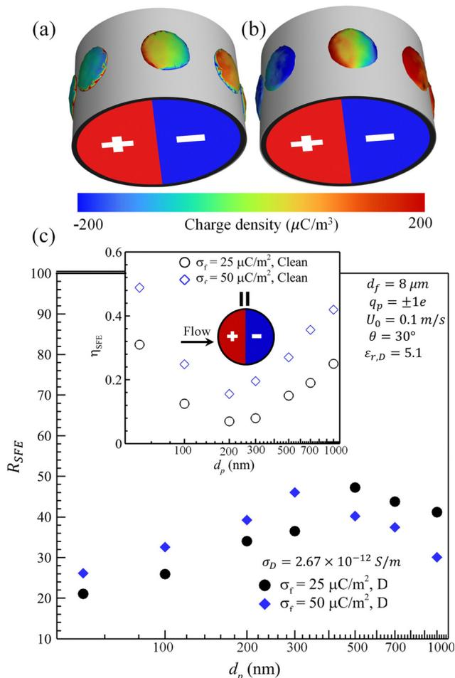
Fig. 5 Volumetric charge density contour plots for DOP droplets deposited on bipolarly charged fibers having surface charge density of  $\sigma_f = 25 \mu\text{C m}^{-2}$  and  $\sigma_f = 50 \mu\text{C m}^{-2}$  are shown in (a) and (b), respectively. SFE reduction due to the DOP loading is shown in (c) with the SFE of the clean fiber shown as the inset. A contact angle of  $30^\circ$  and a surface tension of  $0.015 \text{ N m}^{-1}$  were considered for the DOP droplets.
