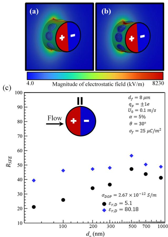
Fig. 6 Contour plots of electrostatic field magnitude around a DOP-loaded charged fiber are shown in (a) and (b) for relative permittivity values of  $\epsilon_{r,D} = 5.1$  and  $\epsilon_{r,D} = 80.18$ , respectively. SFE reduction due to the DOP loading is shown in (c) which is relative to the data of clean fibers shown as the inset in Fig. 5c for  $\sigma_f = 25 \mu\text{C m}^{-2}$ . In this figure, the fiber has a parallel dipole.
