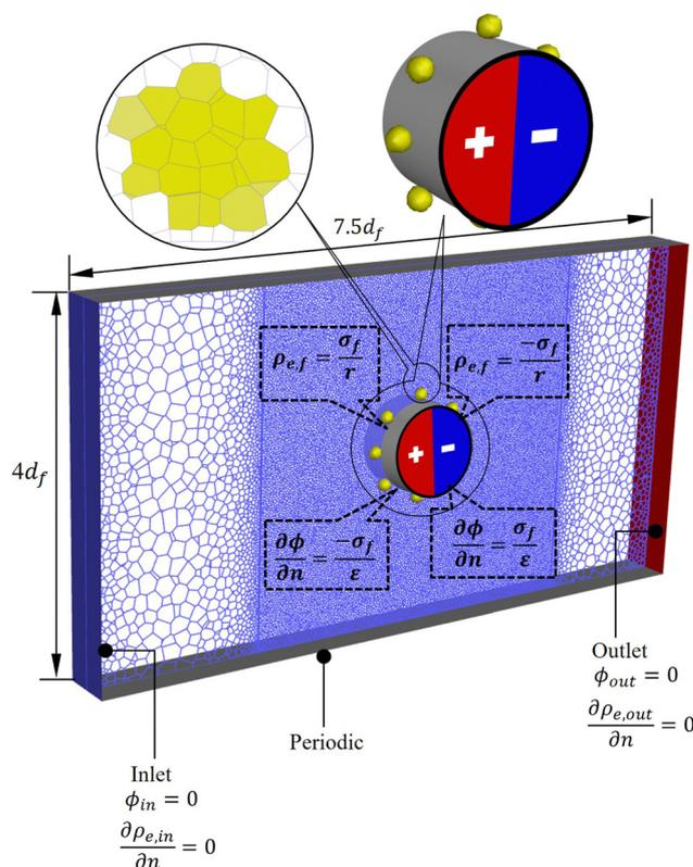
Fig. 1 Computational domain and its boundary conditions. The yellow-filled cells represent the droplets at time zero.
