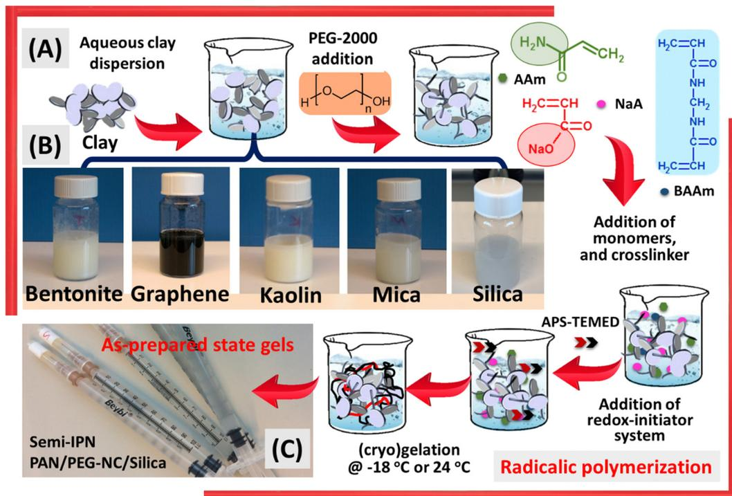
**Scheme 1** (A) Synthetic steps performed during preparation of hybrid PAN/PEG-NC gels. (B) Aqueous dispersion of bentonite, graphene, kaolin, mica and silica. (C) Polypropylene syringes containing silica-filled hybrid gels after completion of the polymerization reaction.
