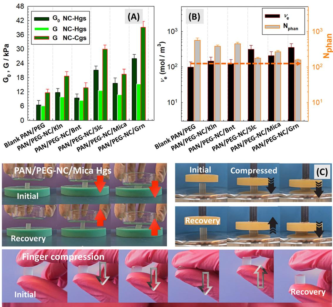
Fig. 4 (A) Comparison of compressive elastic moduli at equilibrium swollen state  $G$  with that of as-prepared state  $G_0$ . (B) Effective crosslink density and network chain length  $N$  of hybrid PAN/PEG-NC gels calculated by phantom network model. (C) Optical views of mica-doped hybrid gels during uniaxial compression and finger testing; before and after removal of stress.
