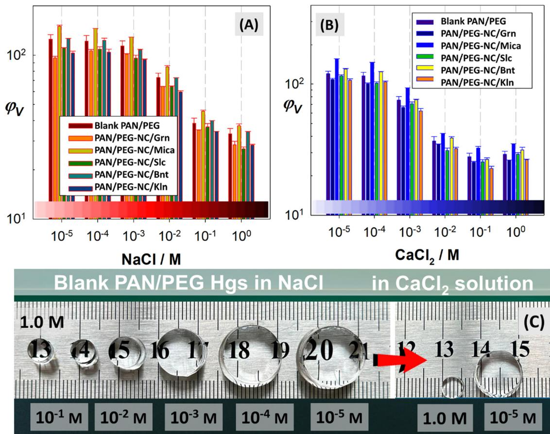
Fig. 7 The equilibrium volume swelling ratio of hybrid hydrogels as a function of the ionic strength of salt solution of NaCl (A) and  $\text{CaCl}_2$  (B), respectively. Optical images of blank PAN/PEG gels in salt solutions of different ionic strengths (C).
