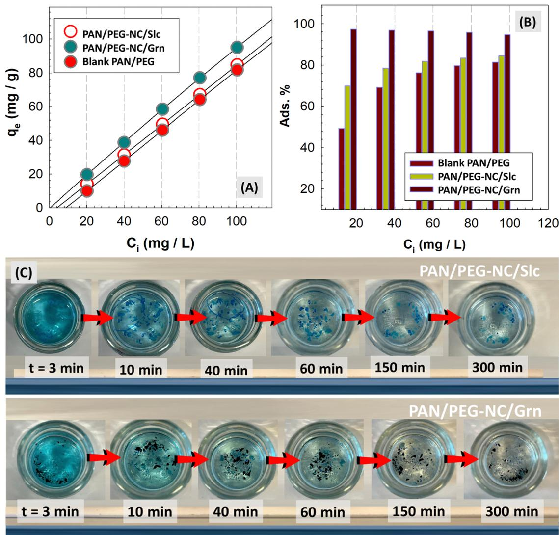
Fig. 10 Adsorption capacity  $q_e$  (A) and adsorption% (B) of hybrid PAN/PEG-NC gels and optical views of Slc and Grn-integrated hybrid gels during adsorption (C). (The fixed experimental conditions: MB concentration: 20–100 mg L<sup>-1</sup>, adsorbent mass: 10 mg,  $V_{\text{dye}} = 20$  mL, time = 24 h, stirring rate = 180 rpm and  $T = 23$  °C.)
