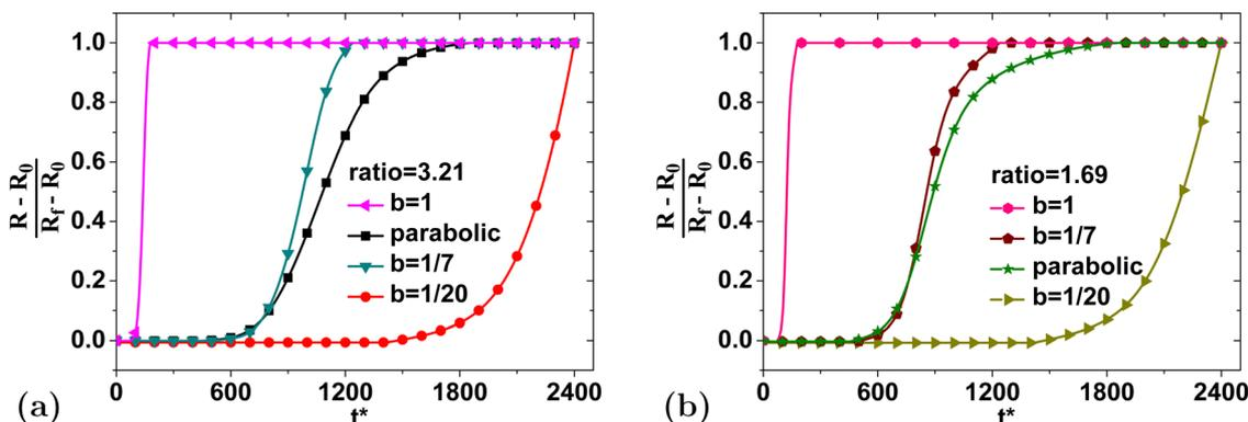
Fig. 14 Comparison of the effect of the heating rate on the functional form of the swelling curve. Note that the parameter  $b$  corresponds to the linear heating ramp  $T = 323 + bt$ , while the parabolic profile refers to heating using eqn (22). The results from two different swelling ratios are shown: (a)  $R_t/R_0 = 3.21$  and (b)  $R_t/R_0 = 1.69$ .
