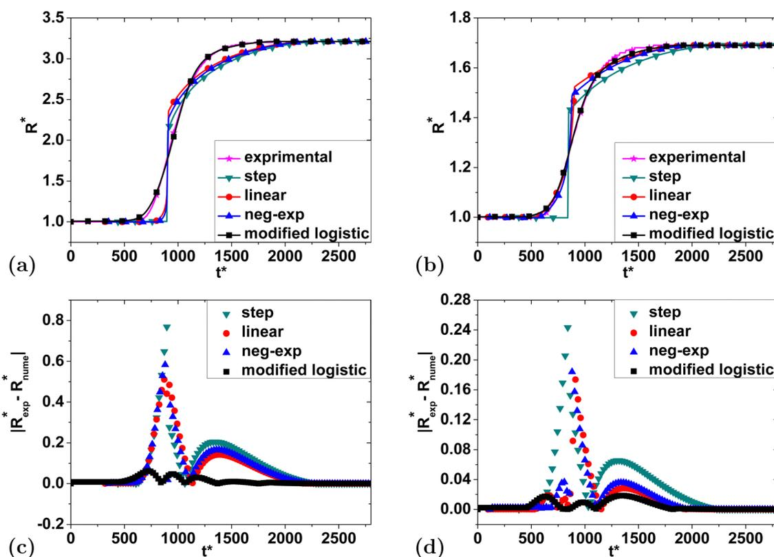
Fig. 4 Comparison of the best fit to the experimental data using the four different empirical models for the two extreme values of the swelling ratio: (a)  $R_f/R_0 = 3.21$  and (b)  $R_f/R_0 = 1.69$ . (c) and (d) show the error between the different models and the experimental data from (a) and (b), respectively.
