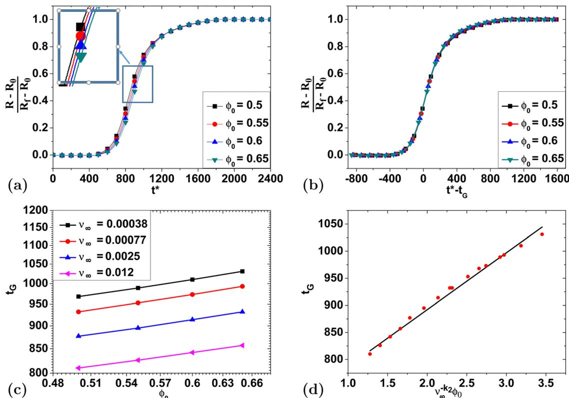
Fig. 9 (a) Swelling curves simulated for various values of  $\phi_0$  for a swelling ratio of 1.69 ( $\nu_\infty = 0.012$ ). (b) Illustration of the collapse of the curves from (a) by changing  $t_G$ . (c) Illustration of the optimal values of  $t_G$  needed to collapse the swelling curves for different values of  $\phi_0$  at different values of  $\nu_\infty$  on log-log axes. (d) Data in (c) collapsed onto a single curve given by eqn (31).
