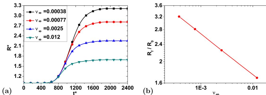
Fig. 8 (a) Swelling curves from Fig. 7(d) replotted to show the impact of  $\nu_\infty$  on the dimensionless radius. (b) Swelling ratio vs.  $\nu_\infty$  on log–log axes.
