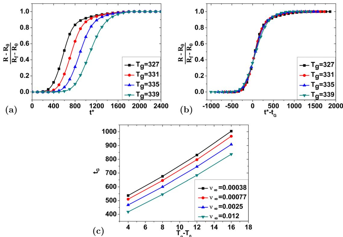
Fig. 10 (a) Swelling curves simulated for various values of  $T_g$  for a swelling ratio of 3.21 ( $\nu_\infty = 0.00038$ ) and initial temperature of 323 K. (b) Illustration of the collapse of the curves from (a) by changing  $t_G$ . (c) Illustration of the optimal values of  $t_G$  needed to collapse the swelling curves for different values of  $T_g$  at different values of  $\nu_\infty$  on linear axes.
