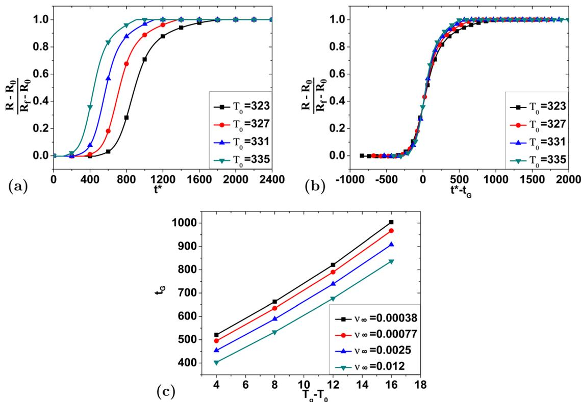
Fig. 11 (a) Swelling curves simulated for various values of  $T_0$  for a swelling ratio of 1.69 ( $\nu_\infty = 0.012$ ) and gelatinization temperature of 339 K. (b) Illustration of the collapse of the curves from (a) by changing  $t_G$ . (c) Illustration of the optimal values of  $t_G$  needed to collapse the swelling curves for different values of  $T_0$  at different values of  $\nu_\infty$  on linear axes.
