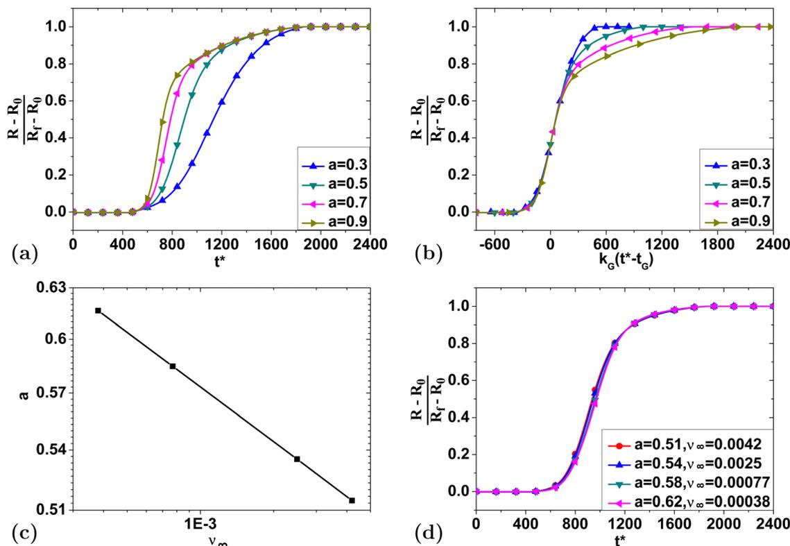
Fig. 7 (a) The swelling curves obtained when  $a$  is varied with all other parameters held constant and the swelling ratio is 1.69 ( $\nu_\infty = 0.012$ ), (b) the best possible rescaling and shifting of the time to collapse the curves in (a). (c) The relation between the optimal value of  $a$  and  $\nu_\infty$  on log–log axes. (d) The swelling curves simulated when  $a$  is varied with  $\nu_\infty$  to produce the best fit to the experimental data.
