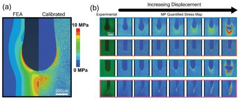
Fig. 6 Quantified stress map using calibration based on MP activation intensity and FEA-derived maximum principal stresses for various fiber end geometries. (a) Side-by-side FEA and calibrated images show stress distribution from experimental intensity data. (b) Calibrated stress maps for different fiber end shapes at various displacement levels. Scale bar in the top left image of (b) applies to all images.
