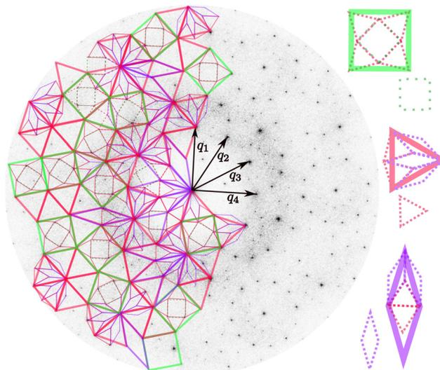
Fig. 3 Analysis of peak positions in the diffraction pattern of Fig. 1(a).  $q_i$  are four basis vectors spanning the reciprocal lattice. Square, triangle, and rhombus tiles are overlaid onto the diffraction pattern. Each tile can undergo further substitution (right side) with irrational inflation factor  $(1 + \sqrt{3})/\sqrt{2}$ . This demonstrates that each diffraction peak position can be written as an integer multiple of the four basis vectors.
