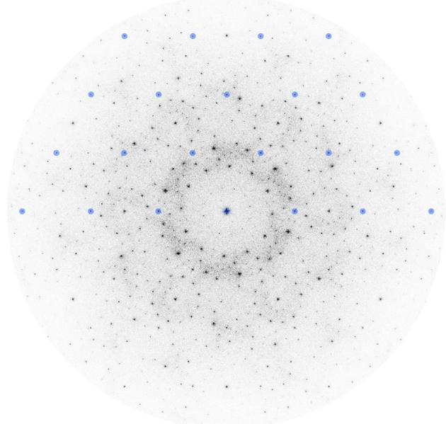
Fig. 6 Simulation snapshot of the six-fold QC at  $T = 0.2$  and  $\varepsilon = 0.5$ . Top: Blue circles represent the minima of the external potential. Bottom: The diffraction pattern, where blue circles representing the reciprocal lattice of the external potential are superimposed on the diffraction peaks.
