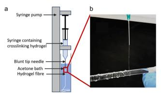
Fig. 2 (a) Experimental set up for spinning hydrogel fibres using a syringe pump (KD Scientific, USA): (b) visual representation of hydrogel filament obtained after spinning 0.5 wt% NaCMC-NaCas solution, 30 minutes after onset of crosslinking (0.4 mL min<sup>-1</sup>, 21G needle, ID 800 μm).
