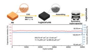
Dense N-doped carbon nanotubes with encapsulated Fe nanoparticles directly grown within red brick as a sustainable monolithic electrode for high-performance supercapacitors
