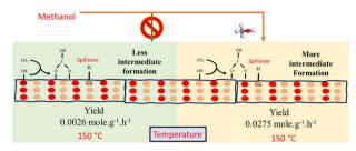
Low-temperature methanol-assisted CO<sub>2</sub> hydrogenation populates intermediates over a Cepromoted Cu/ZnO/MgO catalyst in a three-phase slurry reactor
