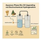
Pinewood and wheat straw bio-oil aqueous phase electrochemical hydrogenation utilising a PtRu/ACC catalyst
