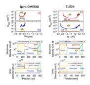
Impact of the hole transport layer on the space charge distribution and hysteresis in perovskite solar cells analysed by capacitance-voltage profiling
