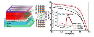
Bulk passivation and suppressing non-radiative recombination loss in a 3D all-inorganic CsPbIBr<sub>2</sub> perovskite solar cell via a 2D layered perovskite framework
