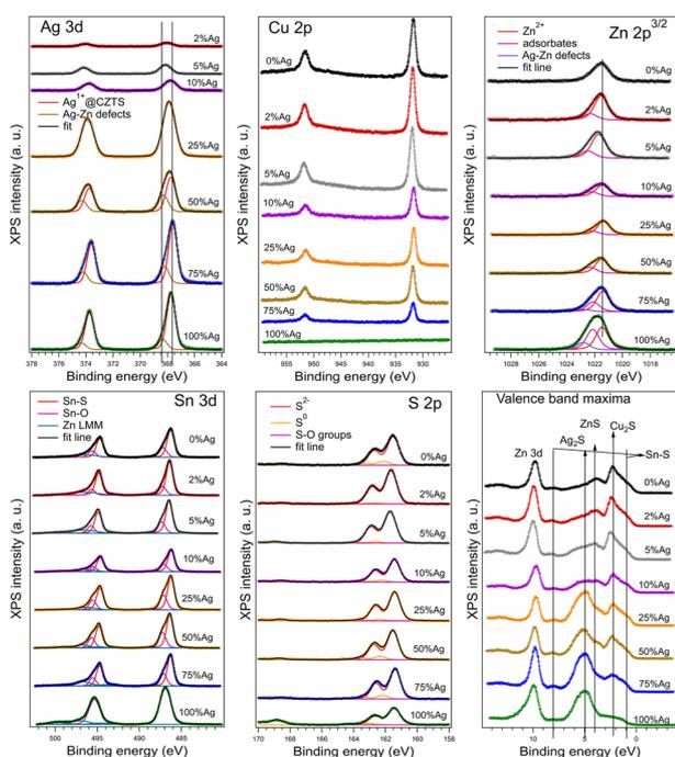
Fig. 8 XPS spectra of CZTS absorber layers with different concentrations of silver: Cu 2p, Ag 3d, Zn 2p<sub>3/2</sub>, Sn 3d and S 2p.
