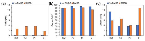
Elemental analysis of used catalysts showing deposition of (a) sulphur, (b) oxygen, and (c) carbon.
