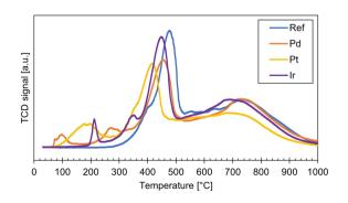
Fig. 3 H<sub>2</sub>-TPR profiles of the reference (ref) Ni-Mo catalyst and the catalysts with Pd, Pt, and Ir, respectively.
