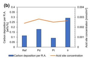
Fig. 7 Carbon deposition on the used catalysts with respect to the relative abundance of non-oxygenated compounds after experiments with (a) no DMDS and (b) DMDS. R.A. is an abbreviation for the relative abundance of non-oxygenated compounds.
