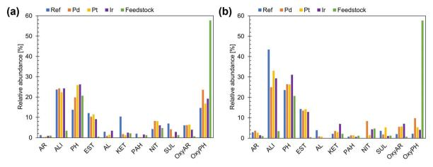
Fig. 4 Classified compounds in the oil after HDO experiments: (a) without DMDS and (b) with DMDS. (AR - aromatics, ALI - aliphatics, PH alkylated phenols, EST – esters, AL – alcohols, KET – ketones, PAH – polycyclic aromatic hydrocarbons, NIT – nitrogen containing compounds, SUL – sulphur containing compounds, OxyAR – oxygenated aromatics, OxyPH – alkoxylated phenols)
