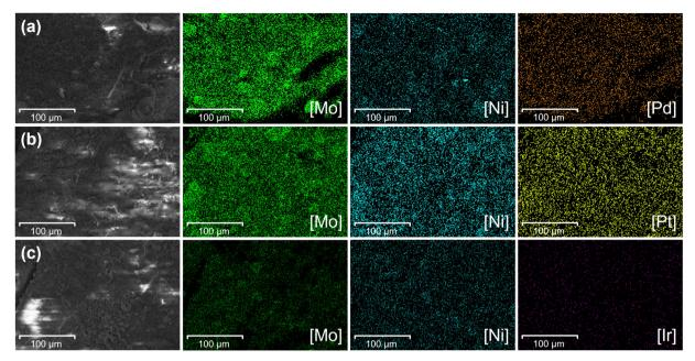
SEM-EDX images for the elemental mapping of catalysts with (a) Pd, (b) Pt, and (c) Ir.
