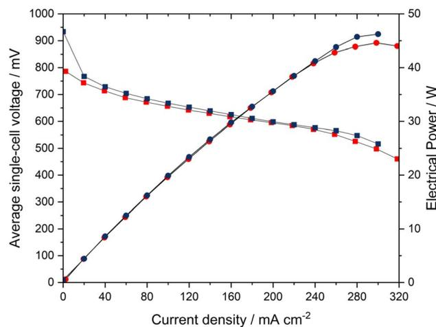
**Fig. 5** Comparison of the  $V$ - $I$  characteristics (squares) and power output (circles) of a HT-PEMFC setup with a 6-cell stack, operated with pure hydrogen (blue symbols) and reformat from the miniplant (red symbols). Fuel cell:  $T = 423 - 443$  K;  $Q_{\text{H}_2} = 800 - 900$  ml min<sup>-1</sup>; 2560 ppm CO, 25% CO<sub>2</sub> in the reformat;  $\lambda_{\text{O}_2} = 2.5$ ; 6 cells with 50 cm<sup>2</sup> active area each.
