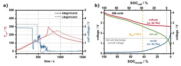
Fig. 2 (a) Trends in cell temperature ( $T_{\text{cell}}$ ) and cell voltage ( $U_{\text{cell}}$ ) for both the SIB- and the LIB-cell, each at an SOC of 30%. (b) Theoretical full cell voltage profile of an SIB, based on the respective half cell curves from the data provided for commercially available HC electrode sheets and NFMO-material in ref. 36 and 37, respectively (n:p-ratio = 1.5:1, assumed initial coulomb efficiency of anode = 90%).
