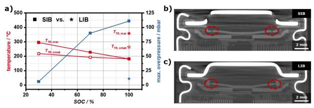
Fig. 3 (a) Summary of the SOC-dependent TR-behaviour, by means of  $T_{\text{TR,onset}}$ ,  $T_{\text{TR,max}}$  and  $p_{\text{max}}$  of the SIB- and LIB-cells investigated. The  $T_{\text{TR,max}}$ -values of the SIB-cells at 70% SOC and 100% SOC are not reasonable due to the strong jelly roll ejection at these SOCs. CT-images of the top of (b) the SIB-cell and (c) the LIB-cell.
