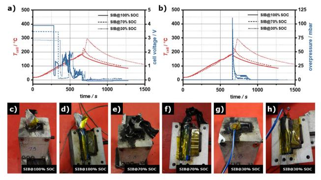
Fig. 1 Trends of (a) cell temperature ( $T_{\text{cell}}$ ) and cell voltage ( $U_{\text{cell}}$ ), and (b)  $T_{\text{cell}}$  and overpressure (p) during the thermal abuse test of the SIB-cells at different SOCs. Photographs of the SIB-cells after the thermal abuse test at (c and d) 100% SOC, (e and f) 70% SOC and (g and h) 30% SOC.
