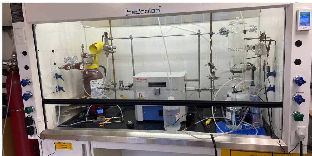
Fig. 3 Ammonia decomposition test setup.
