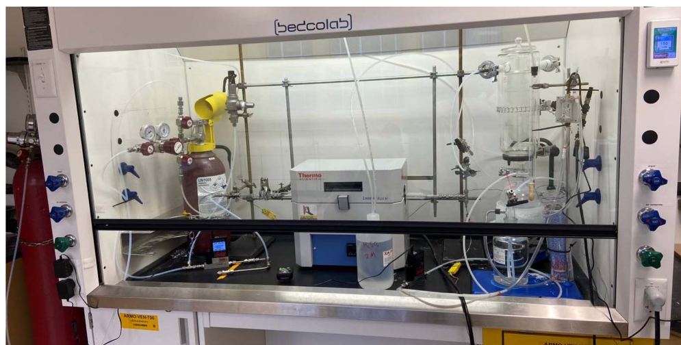
Fig. 3 Ammonia decomposition test setup.
