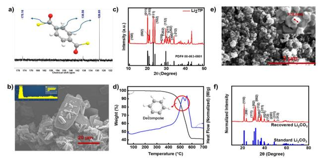
Fig. 5 (a) <sup>13</sup>C NMR for extracted solution, (b) the morphology of recrystallized Li<sub>2</sub>TP, (c) the structure of recrystallized Li<sub>2</sub>TP, (d) TGA for recrystallized Li<sub>2</sub>TP, (e) the morphology of recovered Li<sub>2</sub>CO<sub>3</sub> (f) the structure of recovered Li<sub>2</sub>CO<sub>5</sub>.
