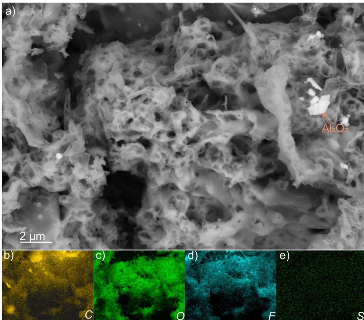
Fig. 4 SEM higher magnification surface morphology and elemental EDX mapping of AA anode sample. (a) surface morphology, (b–e) elemental mapping of carbon, oxygen, fluorine and silicon respectively.
