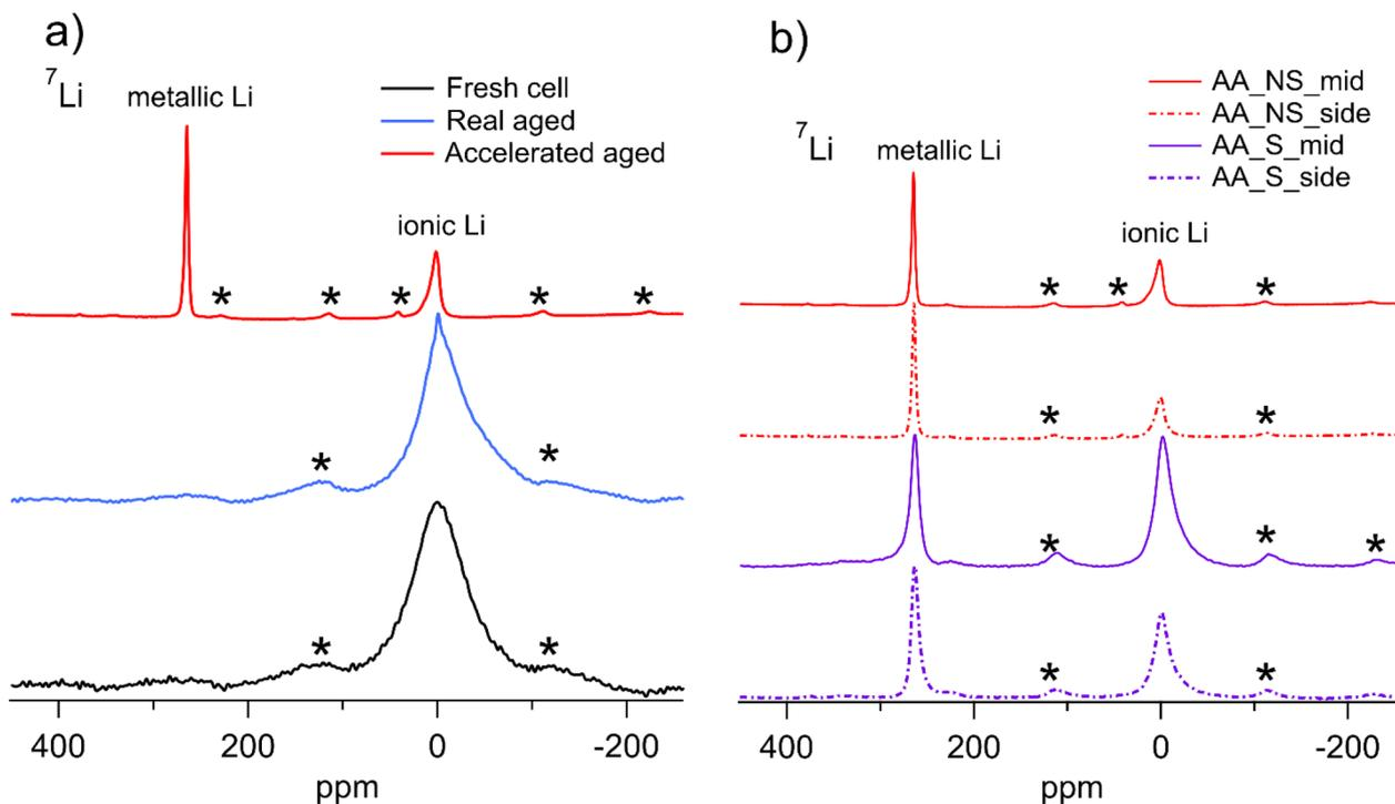
Fig. 2  $^7\text{Li}$  MAS NMR spectra. (a) Comparison of fresh, real life aged (RA) and accelerated aged (AA) cell, (b) AA cells with different storage history and sample position. The “S” letter indicates cells that after accelerated ageing were stored for 11 weeks while “NS” indicates non-stored cells, *i.e.* cells that were opened the same day after the accelerated ageing was completed. The lines marked with asterisks reflect spinning side bands.
