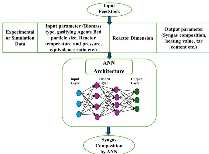
Fig. 10 Flow diagram of data driven modeling.
