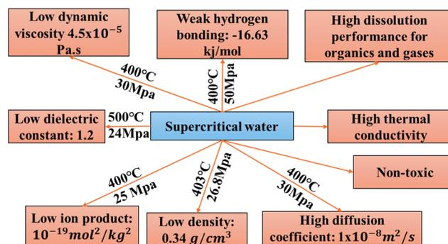
Fig. 6 Unique physicochemical properties of supercritical water.
