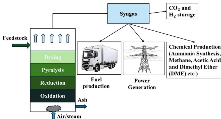
Fig. 1 Basics of gasification process and its applications.
