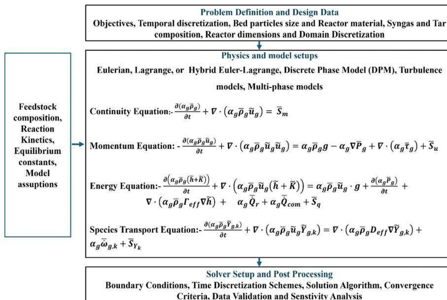
Fig. 9 Mapping data flows for gasification CFD models.
