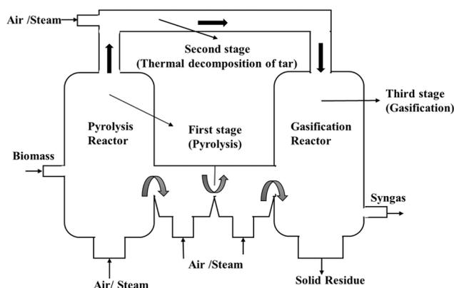
Fig. 5 Line diagram of multistage gasifier.<sup>53</sup>
