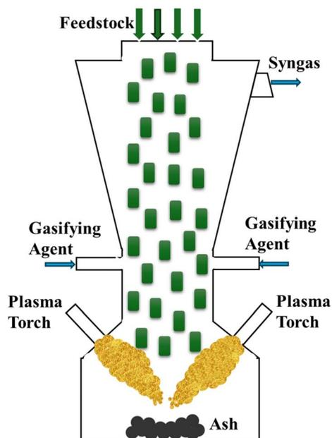
Fig. 4 Schematic diagram for plasma gasification reactor.
