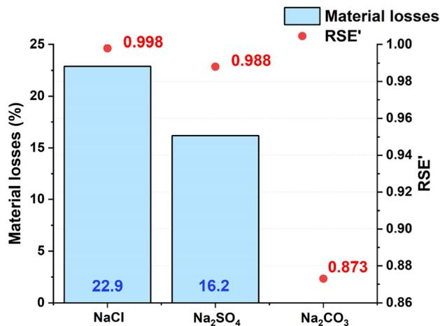
Fig. 3 Material losses due to corrosion and  $RSE'$ .
