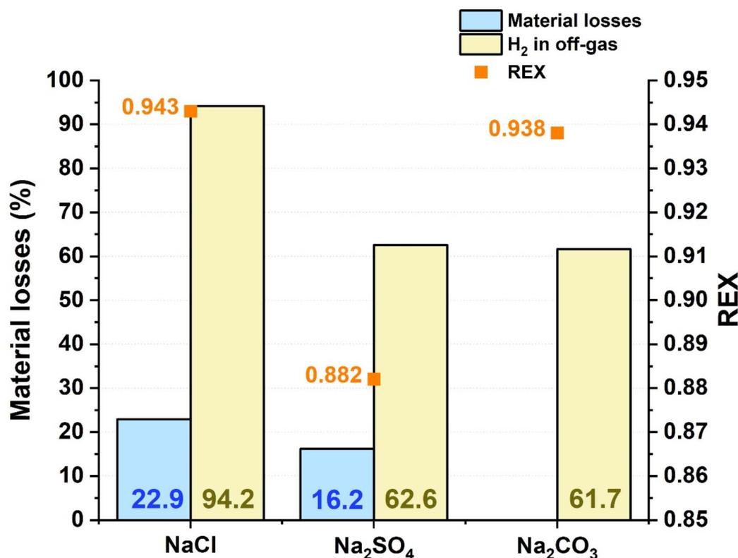
Fig. 5 Relative exergy content (REX), material losses due to corrosion (%), and  $H_2$  vol% in off-gas.
