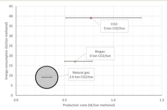
Fig. 5 Overview of production costs (x-axis), energy consumption (y-axis) and  $CO_2$  emission (bubble size, also indicated in text) of the evaluated methanol production routes at 50 € per MWh. The error bars show the possible production costs at 25 € per MWh and 100 € per MWh for each production route.
