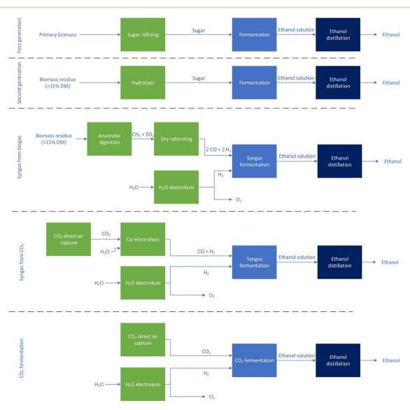
Fig. 2 Overview of evaluated ethanol fermentative production routes: the conventional route based on sugar cane; a second-generation based route, a biogas-based route, a syngas from CO<sub>2</sub> fermentation route, and a direct CO<sub>2</sub> fermentation route.
