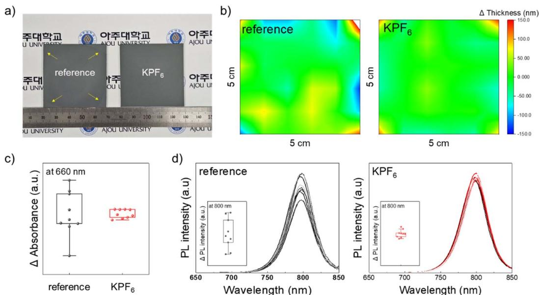
Fig. 5 (a) Optical image of the large-area perovskite films (yellow arrows: inhomogeneous region on the perovskite films). (b) Thickness uniformity of a  $5 \times 5$  cm<sup>2</sup> size perovskite film. (c) Absorbance uniformity test of the large-area perovskite film by UV-Vis absorption at 660 nm. (d) PL spectra of 9 pieces cut from a large-area perovskite sample with and without KPF<sub>6</sub>.
