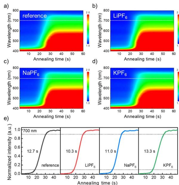
Fig. 1 (a) *In situ* UV-Vis absorption spectra of the perovskite intermediate state for (a) reference, (b) LiPF<sub>6</sub>, (c) NaPF<sub>6</sub>, and (d) KPF<sub>6</sub> during the annealing process. (e) Line profile of UV-Vis absorption intensity at a wavelength of 700 nm. The black dashed lines correspond to 10% and 90% of crystallization during the annealing process, respectively.
