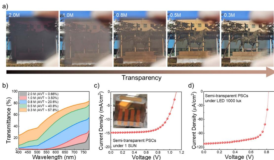
Fig. 6 (a) Photograph images of antisolvent-free perovskite films. (b) Transmittance spectra of the perovskite films with different molar concentrations.  $J$ - $V$  curve of PSCs with semi-transparent perovskite films under (c) 1 sun and (d) LED 1000 lux illumination. The inset shows a photograph of PSCs incorporating a transparent perovskite layer.
