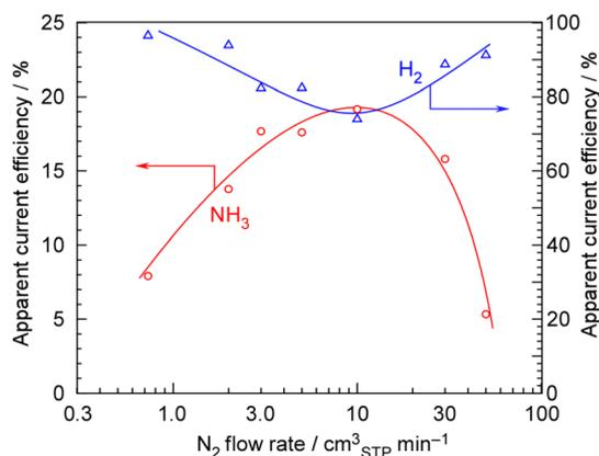
Fig. 4 Apparent current efficiency for  $\text{NH}_3$  and  $\text{H}_2$  formation from  $\text{H}_2\text{O}$  and  $\text{N}_2$  at  $250\text{ }^\circ\text{C}$  and  $1.0\text{ MPa}$  as a function of the  $\text{N}_2$  flow rate for one-pass experiments without  $\text{NH}_3$  separation and unreacted gas recirculation. The anode gas was the mixture of Ar at  $10\text{ cm}_{\text{STP}}^3\text{ min}^{-1}$  with  $5\text{ }\mu\text{L min}^{-1}$  of liquid  $\text{H}_2\text{O}$ .
