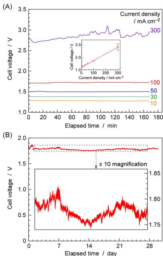
**Fig. 8** Time courses of cell voltage at various current densities (A) and cell voltage changes over several weeks of operation at  $100 \text{ mA cm}^{-2}$  (B) for  $\text{NH}_3$  synthesis and  $\text{H}_2$  formation from  $\text{H}_2\text{O}$  and  $\text{N}_2$  at  $250^\circ\text{C}$ . The inset of (A) shows the relationship between current density and cell voltage. The error bar at  $300 \text{ mA cm}^{-2}$  in (A) represents three times the standard deviation of the data fluctuation.
