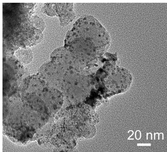
Fig. 9 Transmission electron microscopy image of the 30 wt%-Ru/Cs<sup>+</sup>/C (Cs<sup>+</sup>/Ru = 1 mol mol<sup>-1</sup>) catalyst.
