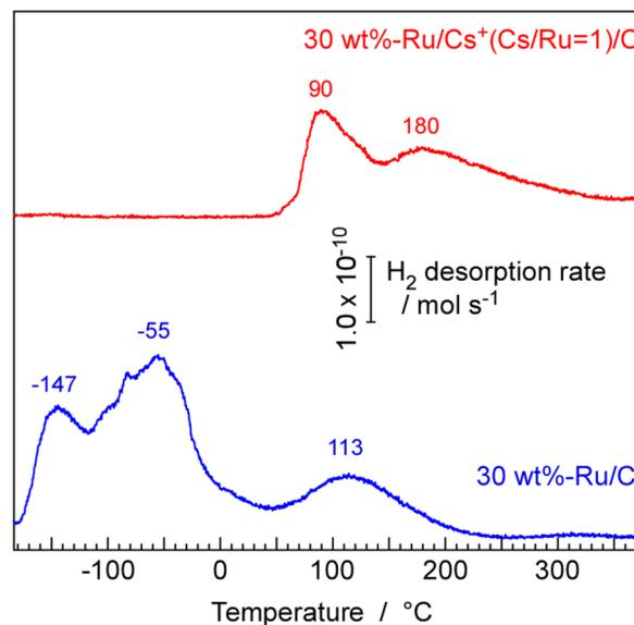
Fig. 10 TPD spectra of H<sub>2</sub> from 30 wt%-Ru/C and 30 wt%-Ru/Cs<sup>+</sup> (Cs: Ru = 1:1)/C. The ramping rate of temperature was 10 °C min<sup>-1</sup>. The samples were treated by reduction treatment at 400 °C, followed by evacuation at 400 °C, prior to TPD measurements. The adsorption of H<sub>2</sub> was performed at -183 °C and 5.0 kPa.
