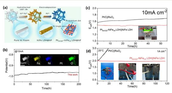
Fig. 7 High current density alkaline water electrolysis: (a) schematic illustration of the synthesis of Pt single atoms and quantum dots on NiFe LDH, (b) chronoamperometric analysis showing long-term stability, (c) long-term stability test for overall water splitting at 10 mA cm<sup>-2</sup>, (d) 1 A cm<sup>-2</sup>. Reproduced with permission from ref. 66 copyright International Journal of Materials Science & Technology, 2025.
