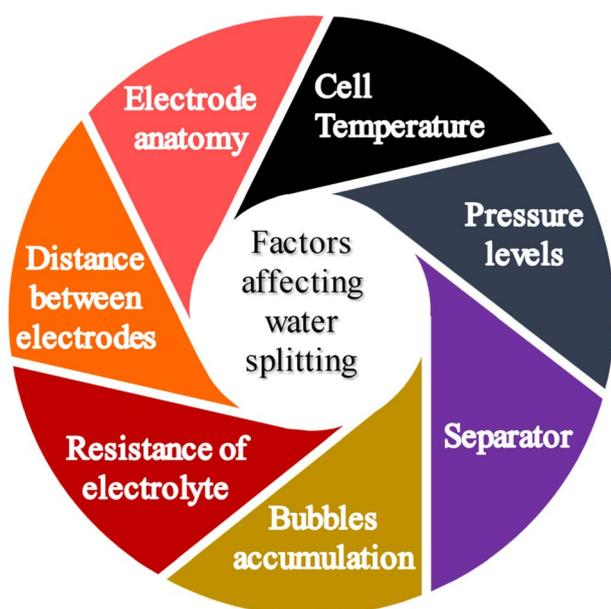
Scheme 1 Factors affecting high current density water electrolysis.
