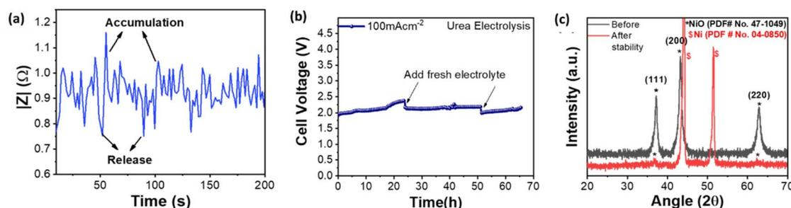
Fig. 10 (a) Dynamic-specific resistance test was performed to examine the evolution of gas bubbles and superhydrophobicity on self-supported nickel foam electrodes. (b) Stability measurement at high current density. (c) Structural stability of the self-supported nickel foam electrodes after 70 h of high current density operation and H<sub>2</sub> evolution. Reproduced with permission from ref. 56 copyright International Journal of Hydrogen Energy, 2024.
