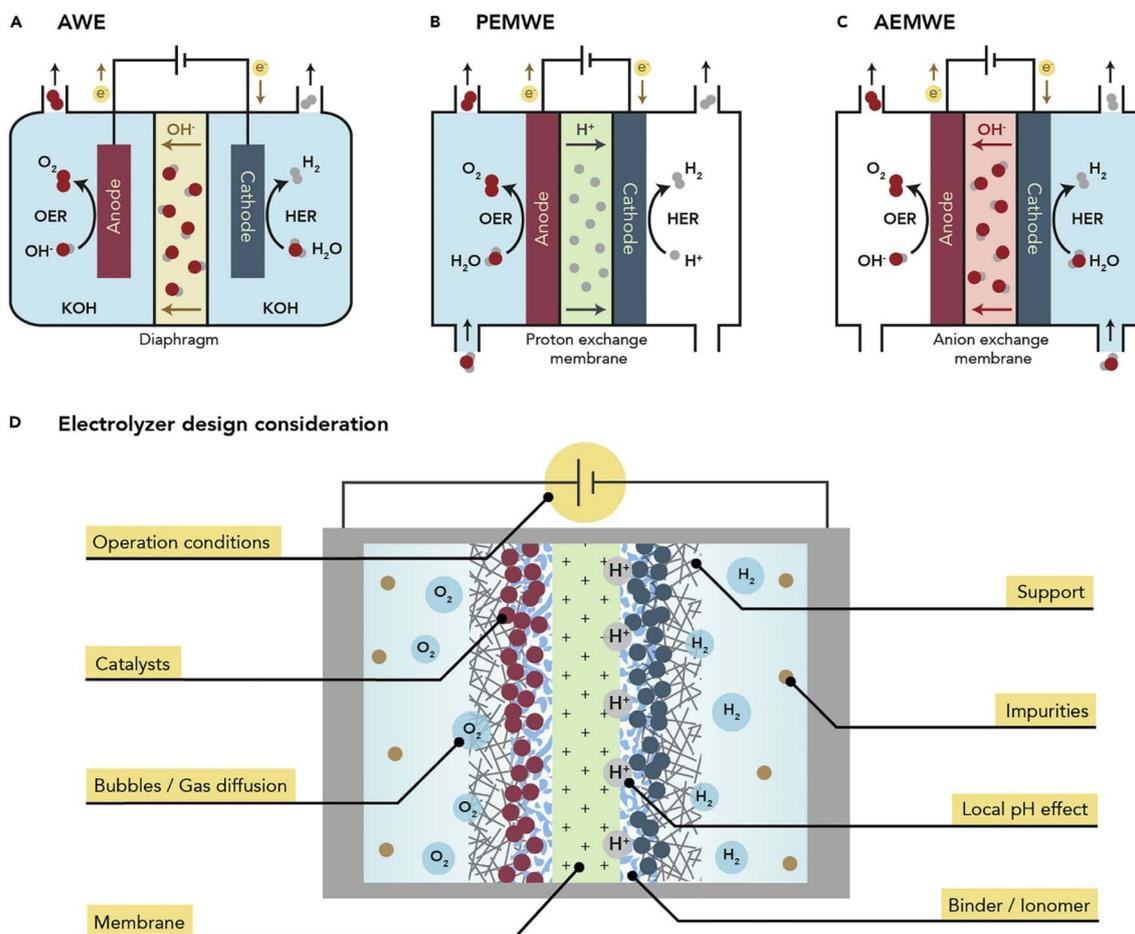
**Fig. 1** Water electrolysis system electrode/electrolyte design configurations: (a) alkaline water electrolyzers (AWE), (b) proton exchange membrane water electrolyzers (PEMWE), (c) alkaline exchange membrane water electrolyzers (AEMWE), (d) key strategies influencing water electrolyzers with for operating in high current density and long-term stability. Reproduced from ref. 10. Copyright the Cell Press, 2021.
