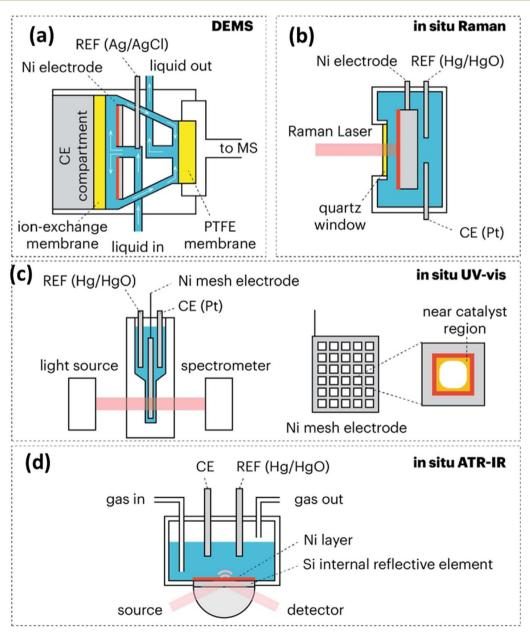
Fig. 11 Illustration of selected *in situ* cell configurations. (a) Differential electrochemical mass spectrometry (DEMS); (b) *in situ* Raman Spectro electrochemistry; (c) *in situ* UV-vis Spectro electrochemistry; (d) *in situ* attenuated total reflectance infrared (ATR-IR) Spectro electrochemistry. Reproduced with permission from ref. 138. Copyright Journal of Catalysis, 2024.
