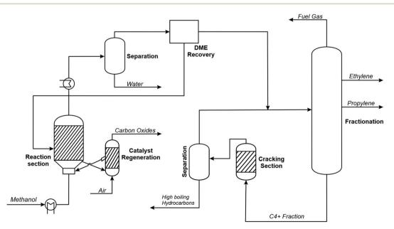
Simplified process flow diagram of the UOP/INEOS MTO process.<sup>243,258</sup>
