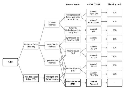
Fig. 1 Main production routes for synthetic jet fuel production.<sup>19</sup>
