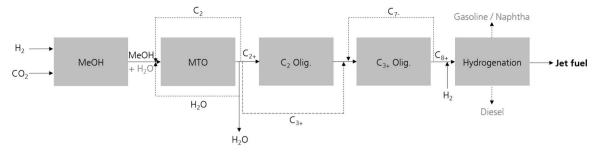
Fig. 11 A simplified block diagram illustrating various recycle options and process configuration discussed in Section 3 regarding the potential for process integration and intensification starting from CO<sub>2</sub> and H<sub>2</sub>.
