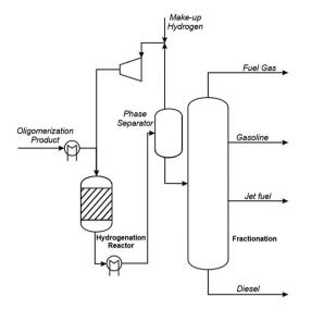
Fig. 10 Simplified process flow diagram of the hydrogenation of the oligomerization products.341
