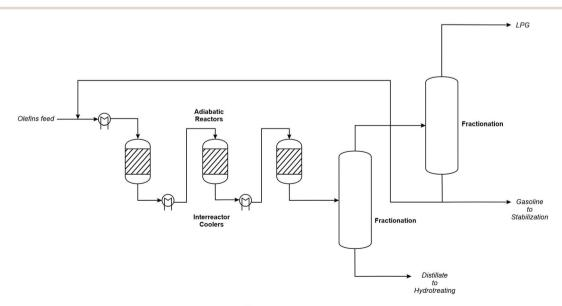
Simplified process flow diagram of the MOGD process.<sup>278</sup>
