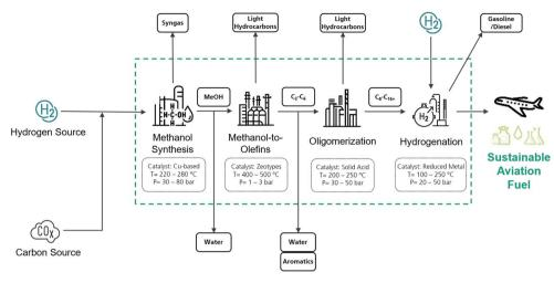
Fig. 2 Sustainable aviation fuel production from hydrogen and carbon source via the methanol pathway. The grey streams represent potential by-products that may occur in the process. 18,56,57
