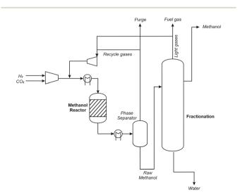
Fig. 3 Simplified process flow diagram of the methanol synthesis. 145
